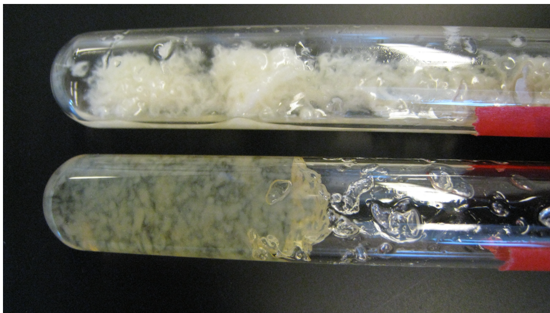
Figure S1. Cellulose precipitated from a 3.7 wt% solution in the IL 1-ethyl-3-methylimidazolium acetate by a 2.5:1 (v/v) of precipitation solvent:cellulose solution with a composition from region (f) (top) and region (b) (bottom) from Fig. 2. Cellulose and biomass precipitated using a solvent composition indicated by region (f) in Fig. 2 are easily filtered and do not form gel phase intermediates during precipitation.
