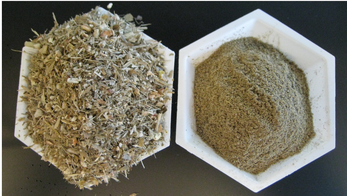
Figure S2. Images of corn stover prior to (left) and after (right) ionic liquid pretreatment. Corn stover particle size is reduced by the pretreatment process and the choice of precipitation solvent and mixing method. Pretreated corn stover in these images was dried under vacuum from an ethanol-wet slurry.
