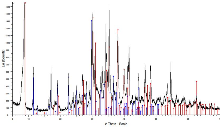
XRD SCAN OF DRIED AQUEOUS PHASE RESIDUE FROM LIGNIN SHOWING THE PRESENCE OF SODIUM CARBONATE AND SODIUM ACETATE
