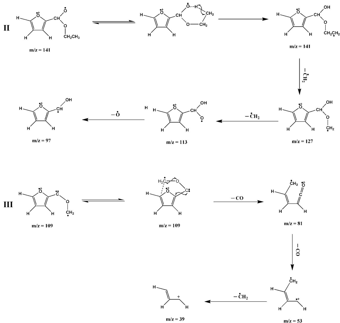
**Scheme S5** Degradation pathway II and III for DEF in GC/MS
