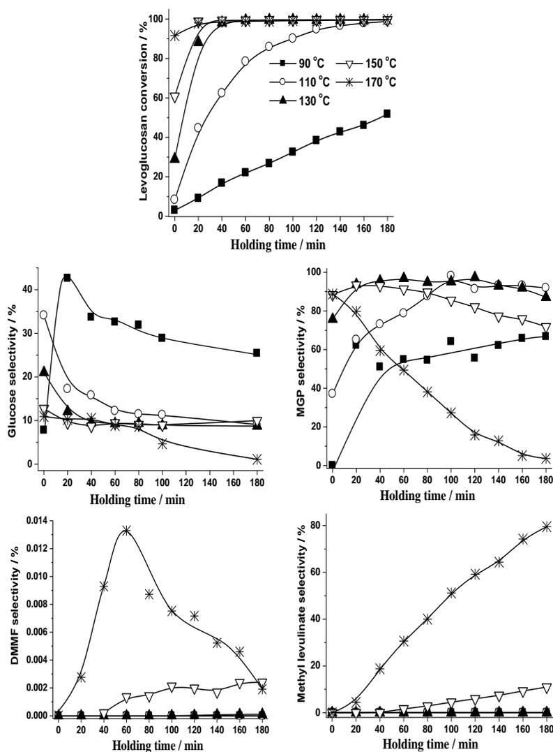
**Fig. S1** Effects of reaction temperature on levoglucosan conversion and product distribution. Methanol/water mass ratio: 4.5; catalyst dosage: 5 wt%; stirring rate: 600 rpm.
