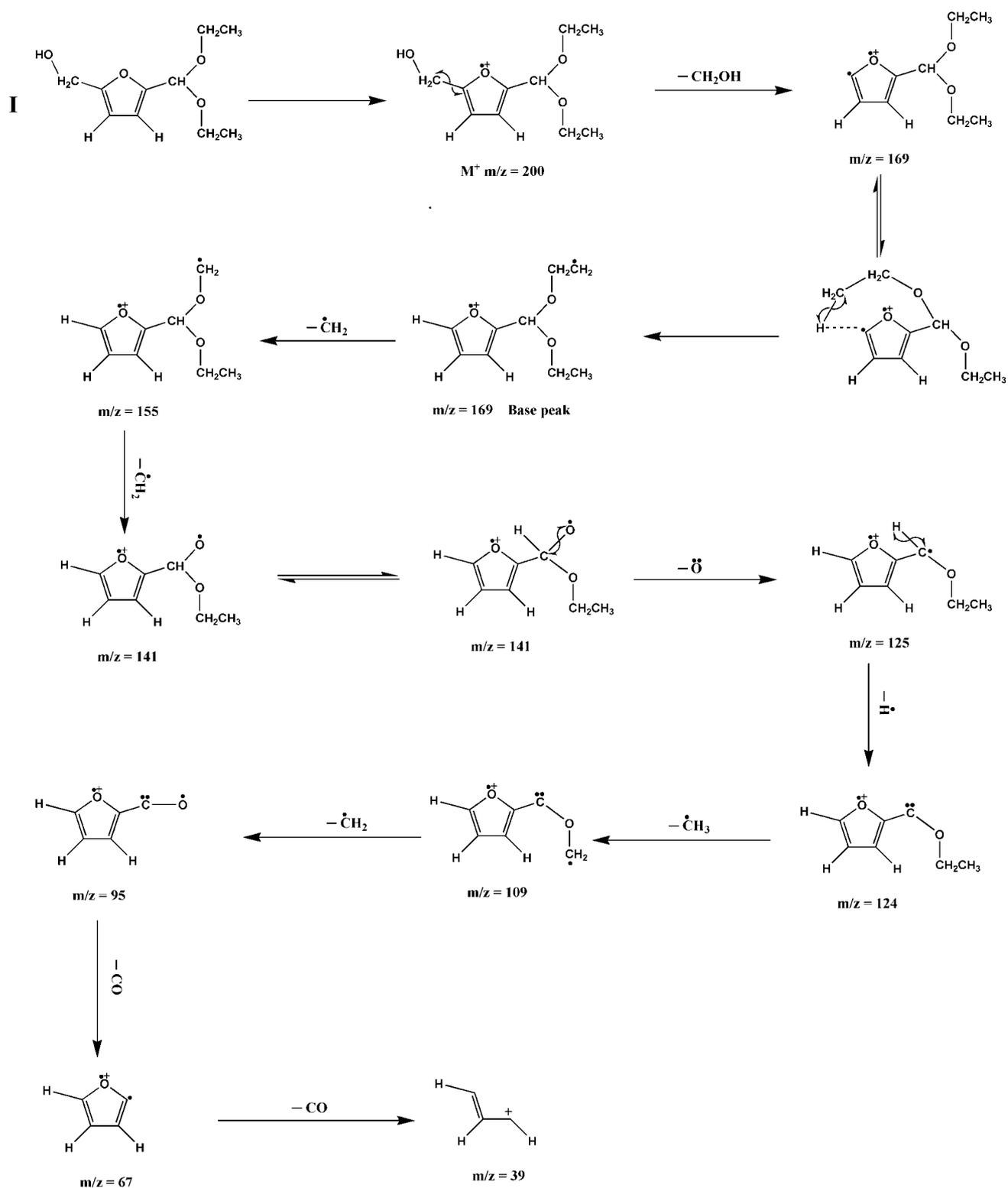
**Scheme S4** Degradation pathway I for DEF in GC/MS
