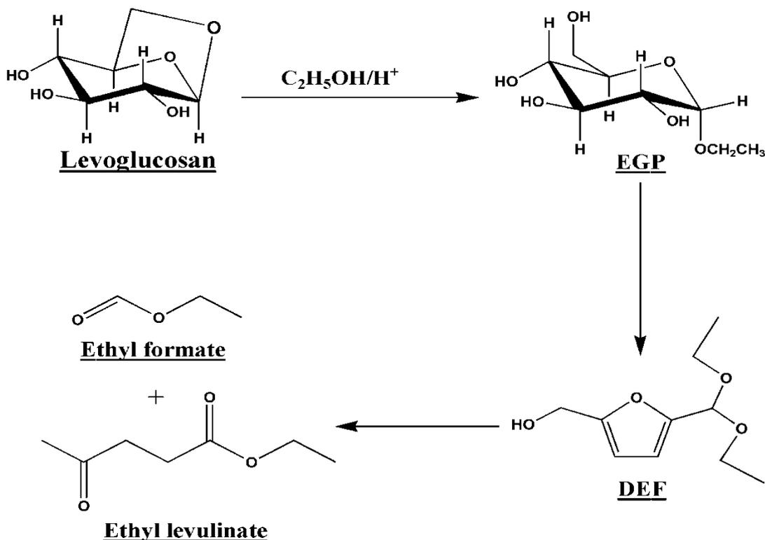
**Scheme S2** Main reaction pathway of levoglucosan in ethanol/water
