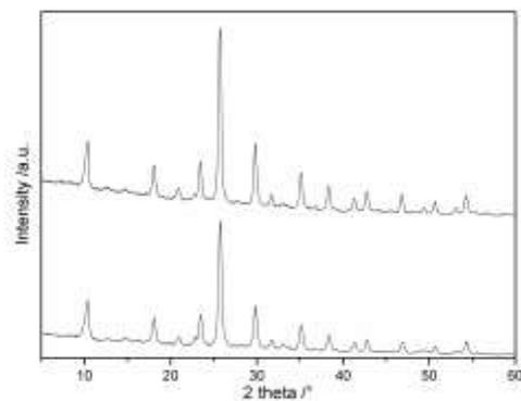
Fig. S5 XRD patterns of CsPW 600°C (lower) and HT CsPW 600°C (upper), showing the influence of hydrothermal treatment
