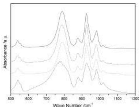
Fig. S1 FTIR spectra from lower to upper:  $\text{H}_4\text{SiW}_{12}\text{O}_{40}\cdot x\text{H}_2\text{O}$ ,  $\text{Cs}_{3.5}\text{H}_{0.5}\text{SiW}_{12}\text{O}_{40}\cdot x\text{H}_2\text{O}$  as prepared,  $\text{Cs}_{3.5}\text{H}_{0.5}\text{SiW}_{12}\text{O}_{40}\cdot x\text{H}_2\text{O}$  300°C and  $\text{Cs}_{3.5}\text{H}_{0.5}\text{SiW}_{12}\text{O}_{40}\cdot x\text{H}_2\text{O}$  600°C.
