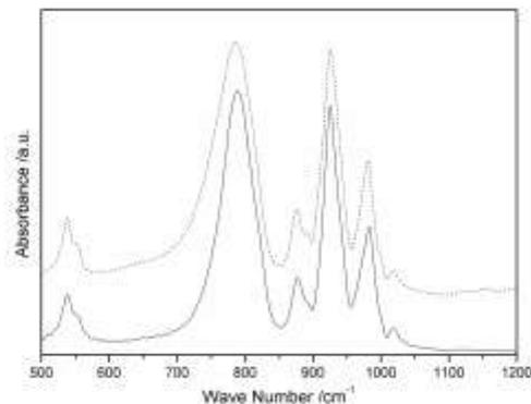
Fig. S3 FTIR spectra of Cs<sub>3.5</sub>H<sub>0.5</sub>SiW<sub>12</sub>O<sub>40</sub>.xH<sub>2</sub>O 600°C before (lower) and after hydrothermal treatment (upper).
