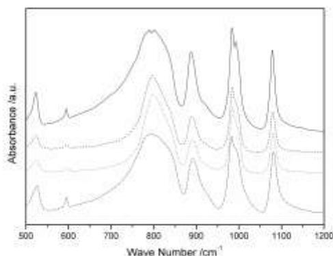
Fig. S2 FTIR spectra from lower to upper:  $\text{H}_3\text{PW}$ , CsPW as prepared, CsPW 300°C and CsPW 600°C.
