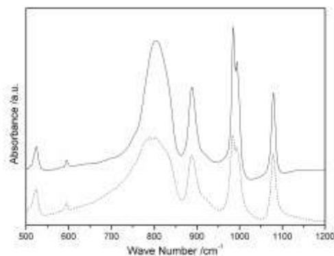
Fig. S4 FTIR spectra of Cs<sub>2.5</sub>H<sub>0.5</sub>PW<sub>12</sub>O<sub>40</sub>.xH<sub>2</sub>O 600°C before (lower) and after hydrothermal treatment (upper).
