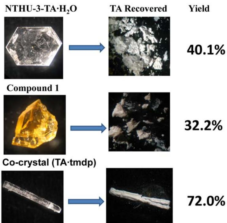
**Fig. S2.** Photos showing TA were recovered from NTHU-3-TA·H<sub>2</sub>O, compound **1** and (TA·tmdp). TA solids remained in solution after the inorganic part was dissolved in 3M HCl solution
