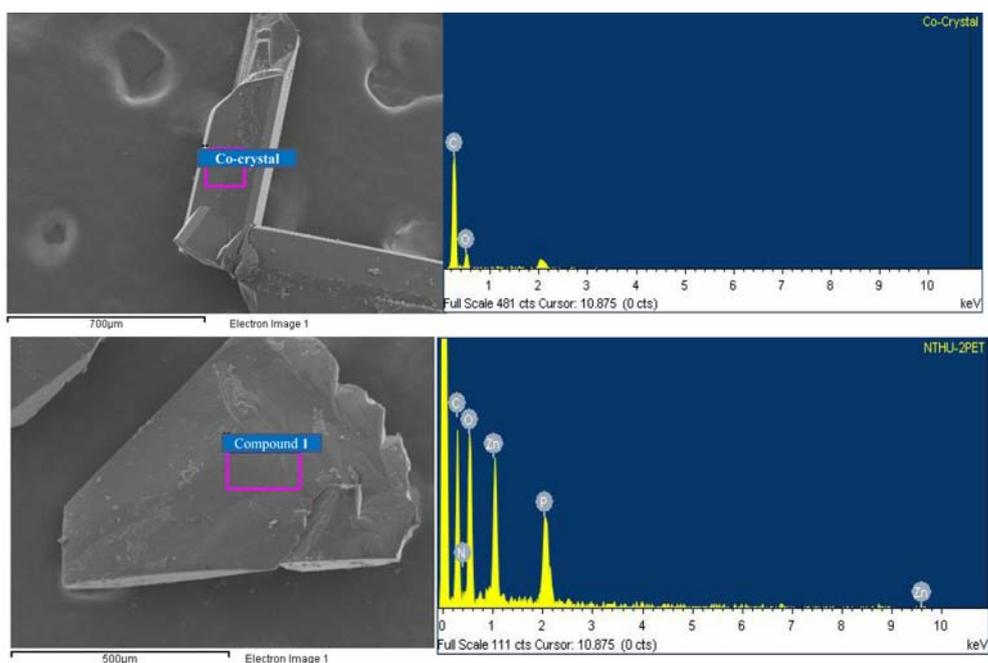
**Fig. S4.** SEM images and EDX spectra for the co-crystals of (TA·tmdp) and compound **1**. Pink rectangles mark the scanned range of electron beam confirming the existing element of Zn, P, O, N, C without impurity elements
