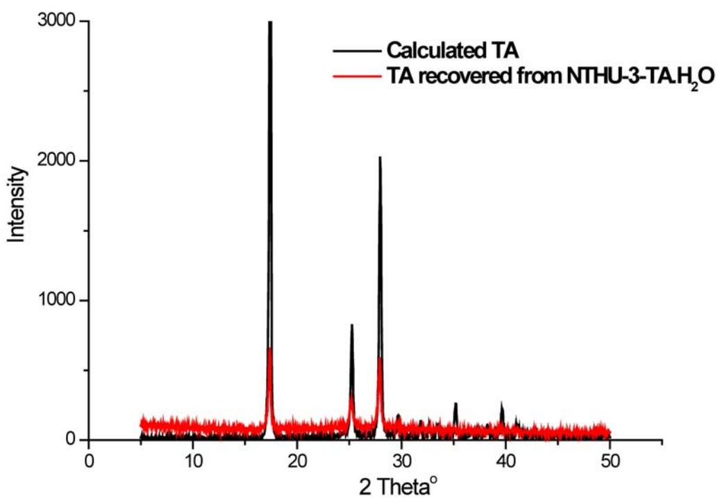
**Fig. S3.** PXRD patterns of TA recovered from NTHU-3-TA·H<sub>2</sub>O.
