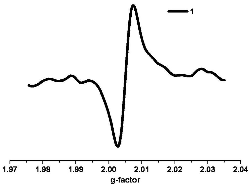
**Fig. S5.** EPR spectrum of compound **1** measured at 298K.
