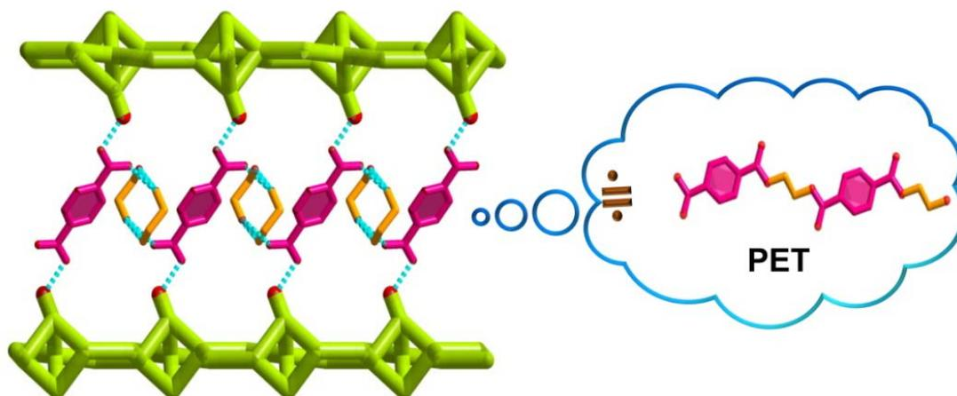
**Fig. S1** The structure of NTHU-3-TA·EG: infinite supramolecular chains of  $\infty\{TA \cdot 2EG\}$  consisting of TA (in pink) and EG (in orange) molecules are residing between zincophosphate layers (in green). The infinite chain was associated with the polymer chain of PET in thinking
