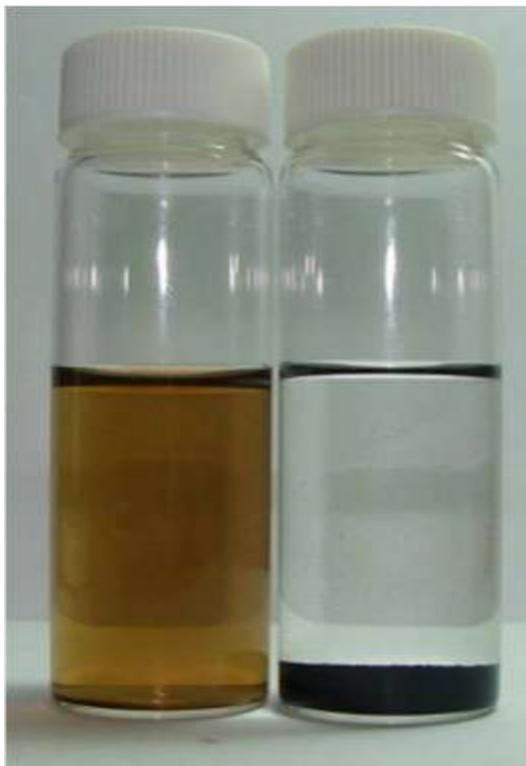
**Fig. S1** GO dispersed in methanol (left) and RGO dispersed in methanol (right). GO dispersion was quite stable in methanol while most of RGO in methanol precipitated at the bottom of the vial.
