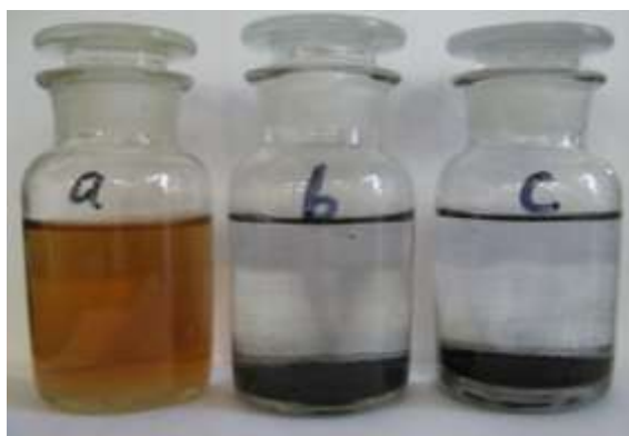
Fig. S3 Comparison of the samples after reaction, reaction condition: microcrystalline cellulose (FMC PH-101, 20-100 mm, 83% crystallinity), 0.5 g; H 2 O, 50 mL; temperature, 518 K; H 2 pressure, 6 MPa at room temperature; 800RPM; a without a catalyst, reaction time, 2 h; b partially conversion of cellulose over Ni/ZnO (0.15 g), reaction time, 0.5 h; c complete conversion over Ni/ZnO, reaction time, 2 h
