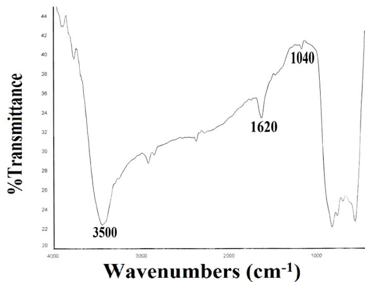
**Figure 6. FTIR spectrum of fresh nano-Al<sub>2</sub>O<sub>3</sub>**
