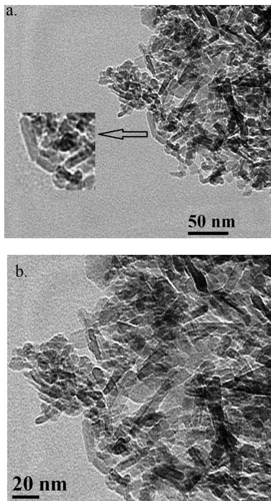
**Figure 4. (a) TEM image of fresh nano- $\text{Al}_2\text{O}_3$  at 50 nm scale (b) TEM image of fresh nano- $\text{Al}_2\text{O}_3$  at 20 nm scale**
