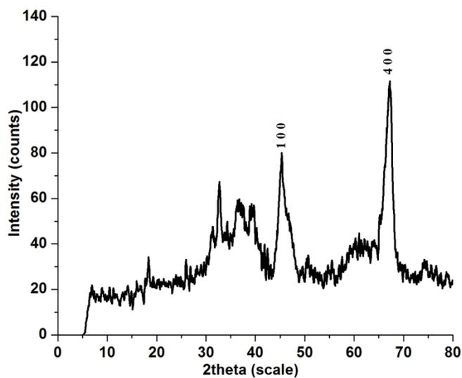
Figure 3. XRD pattern of fresh nano- Al<sub>2</sub>O<sub>3</sub>
