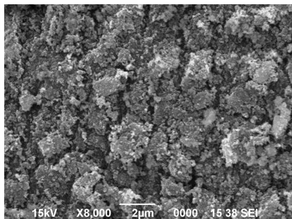
Figure 1. SEM photograph of fresh nano-Al<sub>2</sub>O<sub>3</sub>
