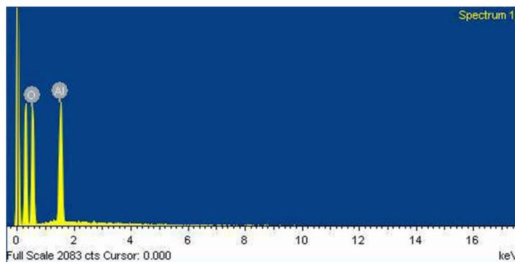
Figure 2. EDX of fresh nano- Al<sub>2</sub>O<sub>3</sub>
