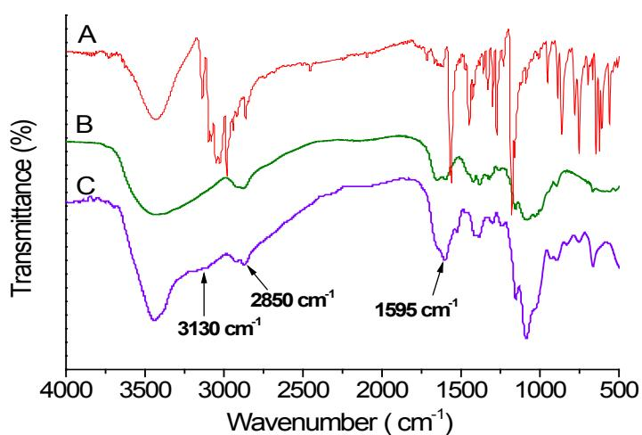
**Fig. 1S** FT-IR spectra comparison of EMImBr (A), CS (B) and CS-EMImBr (C).
