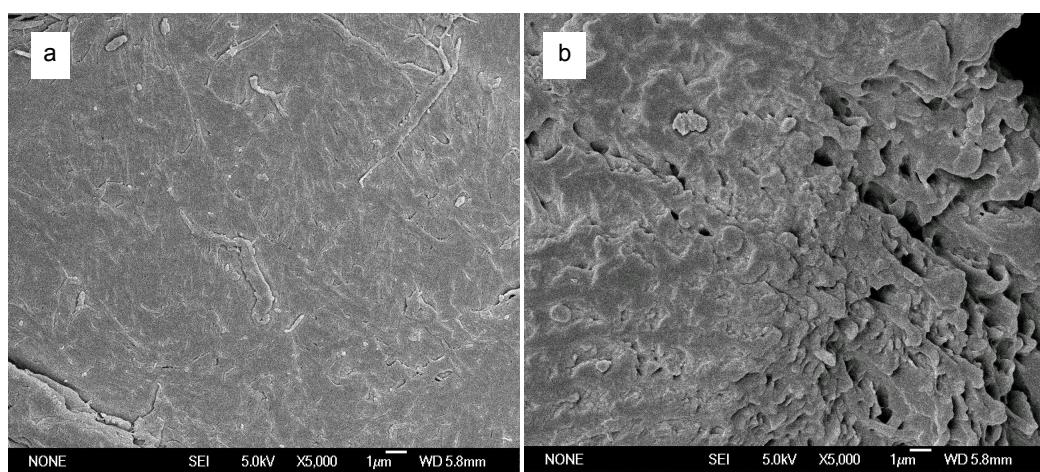
**Fig. 2S** Scanning electron microscopy images of CS (a) and CS-EMImBr (b).
