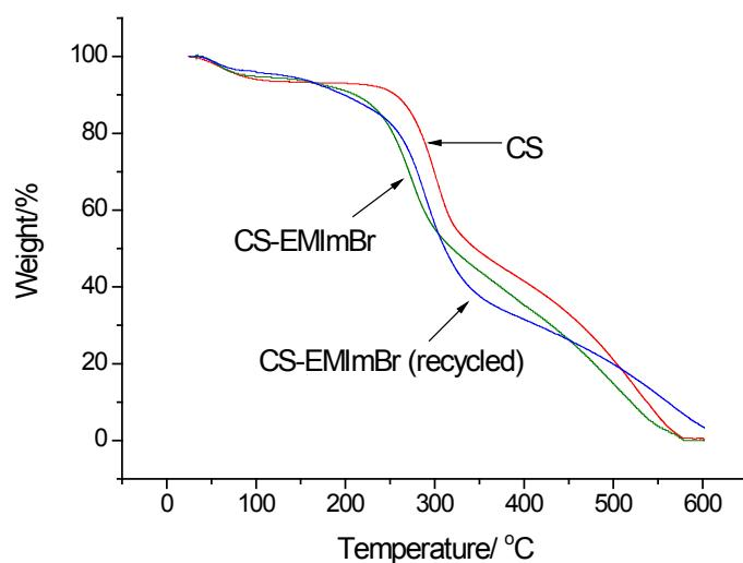
**Fig. 3S** Thermogravimetric curves for CS, CS-EMImBr and four times recycled CS-EMImBr.
