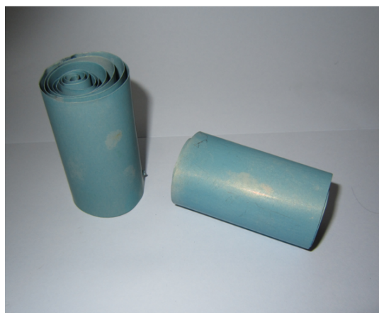
Fig. S1 Photograph of the CoPcS/MMO structured catalyst.
