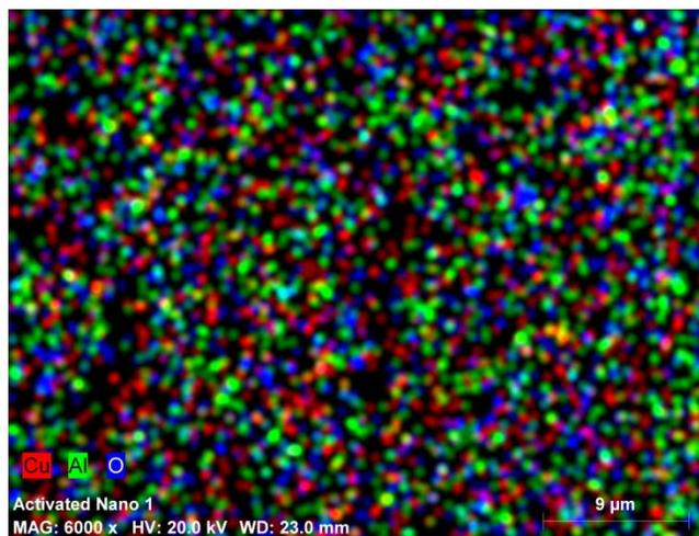
**Fig. 7** EDX of Cu-Al catalyst.
