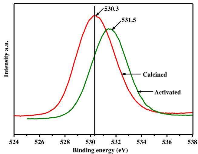
**Fig.2** O 1s spectra of the calcined and activated Cu-Al catalyst.
