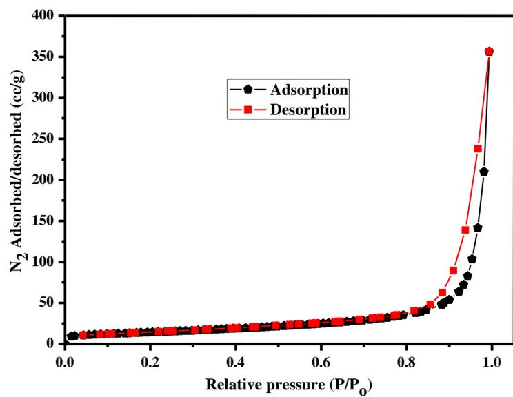
**Fig.1** N<sub>2</sub> adsorption/desorption isotherm of activated Cu-Al catalyst.
