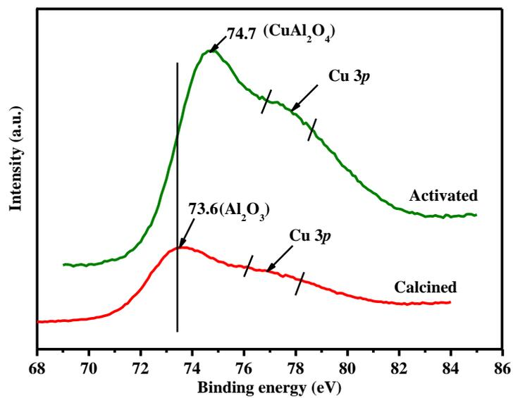
**Fig. 3** Al 2p spectra of the calcined and activated Cu-Al catalyst.
