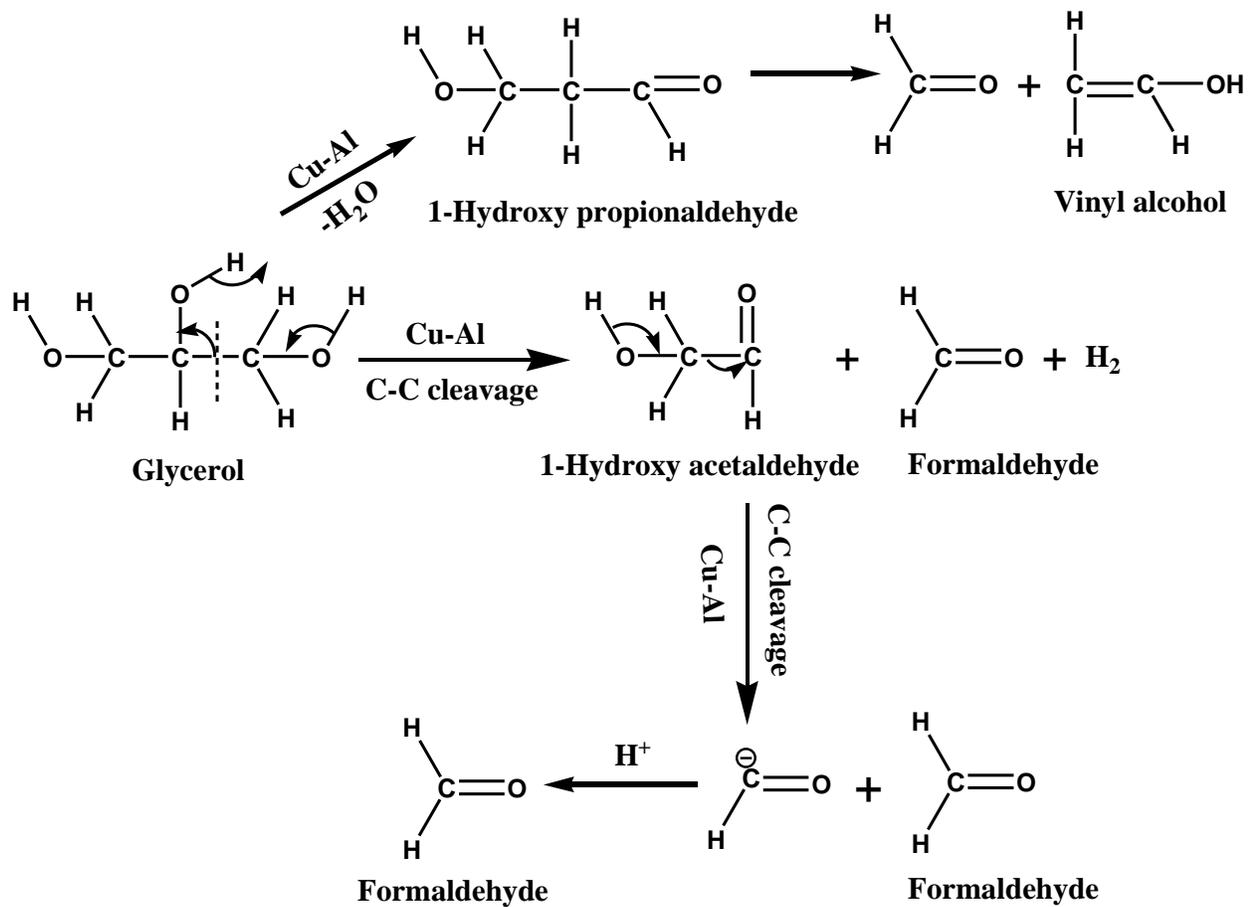
**Scheme 1** Formaldehyde formation by C-C cleavage of glycerol under dehydration condition
