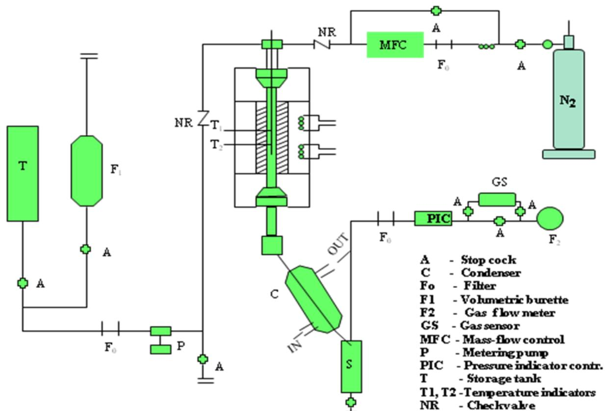
**Fig. 9** Schematic of a continuous fixed bed reactor set-up.
