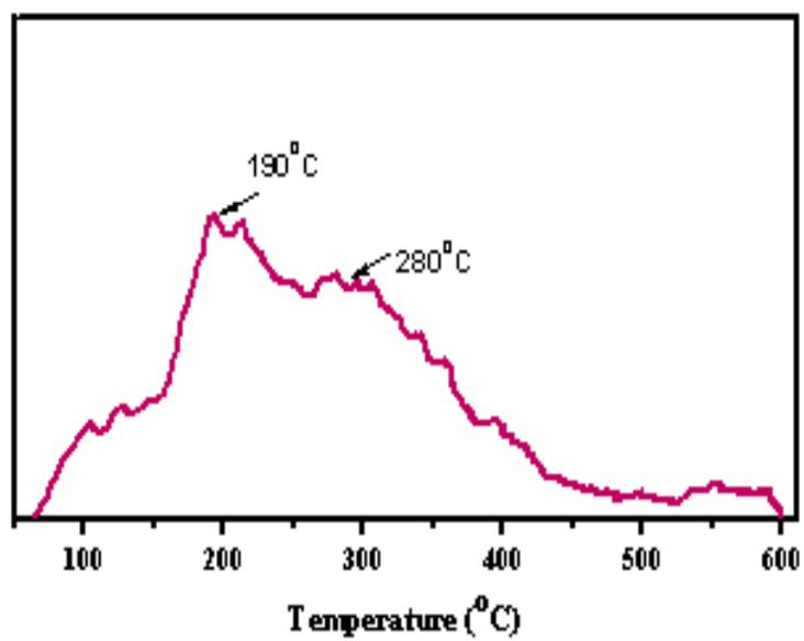
**Fig. 4** CO<sub>2</sub>-TPD profile of the activated Cu-Al catalyst.
