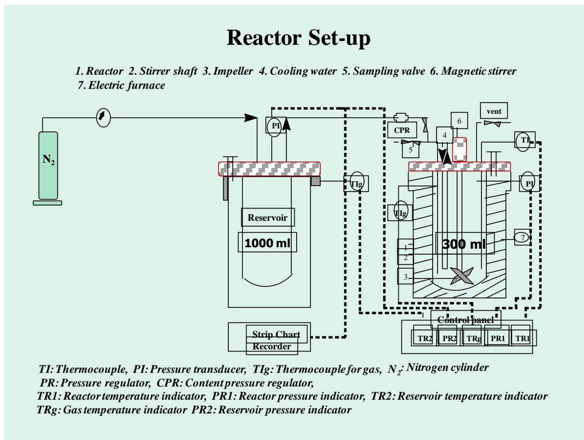
**Fig. 8** Schematic of a batch reactor set-up.
