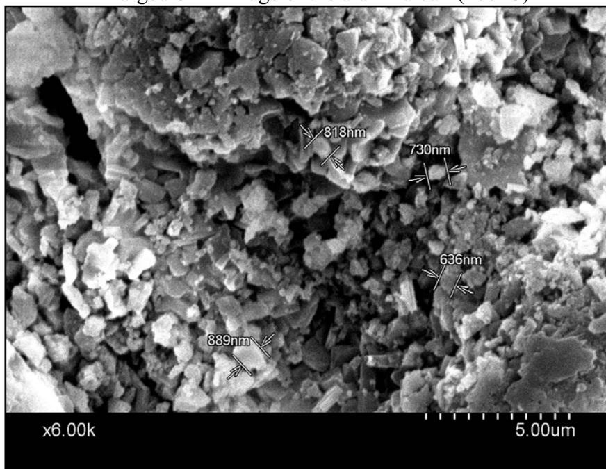
Enlarged SEM image of the alumina ball (700°C)
