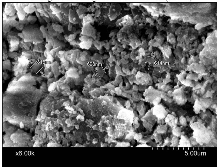
Enlarged SEM image of the alumina ball (400°C)
