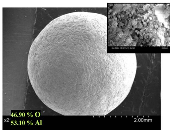
**Figure S1** SEM image of the whole alumina ball; Inset: close-up SEM image of the alumina ball before calcination. The SEM images of an activated alumina ball show aggregates of particles and the highly porous nature of the catalyst (inset). The self-aggregated particle size before calcination is 99-175 nm (evident by enlargement of the inset SEM image).
