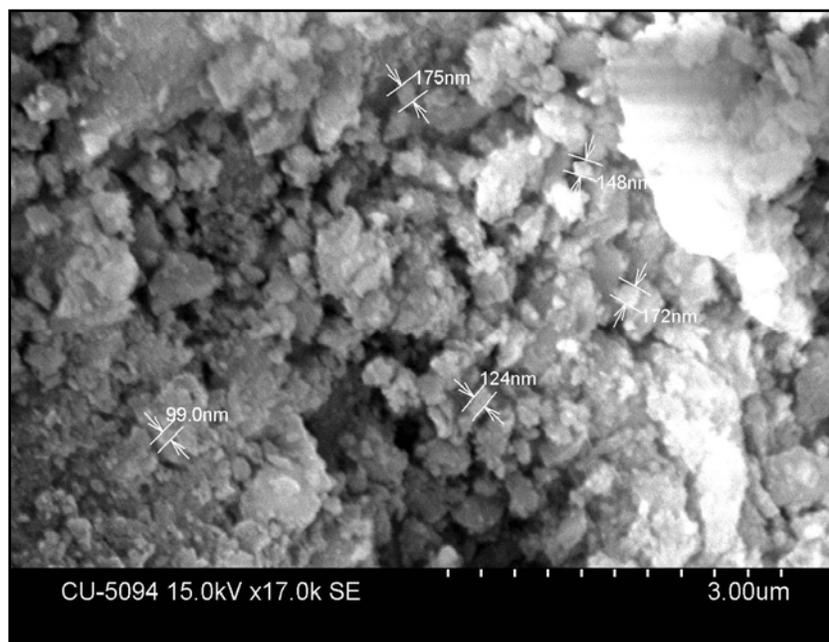
Enlarged SEM image of the alumina ball (120°C)
