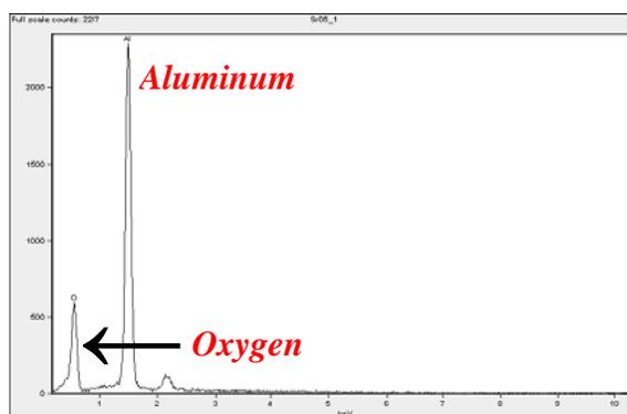
**Figure S4** EDS X-ray spectrum of an activated alumina ball.
