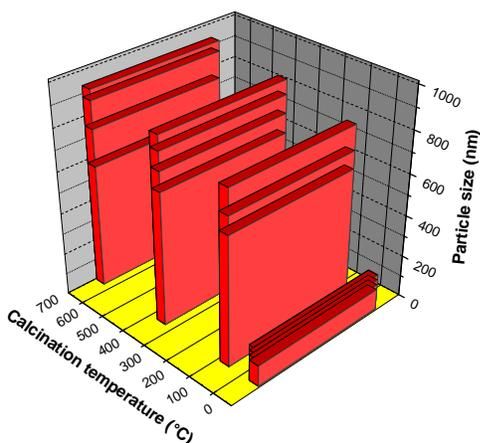
**Figure S3** Change in particle size aggregates with increase in calcination temperature of the activated alumina ball catalyst.
