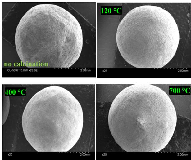
**Figure S2** Clockwise from top left: The SEM images of an activated alumina ball before calcination and after calcination at 120 °C, 400 °C and 700 °C. There is no visible change of the alumina ball to the naked eye, but the close-up high resolution SEM images show that significant morphological changes have occurred on calcinations to 120 °C, 400 °C and 700 °C (given below).
