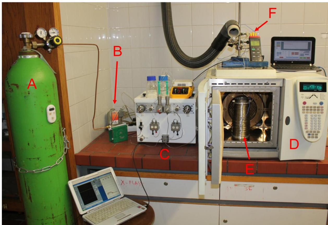
**Fig. S1: Gas-liquid continuous flow reactor.** The main parts of this custom-built device are a gas bottle (synthetic air, 5.0 quality) with a 50 bar pressure regulating valve (A), a mass flow controller (B),<sup>S1</sup> a binary pumping module (C),<sup>S2</sup> a GC oven (D) to heat the residence time unit (E) and a digital 4-channel-thermometer equipped with three thermocouples (F) to monitor the reaction temperature at different positions of the reaction coil.<sup>S3</sup>
