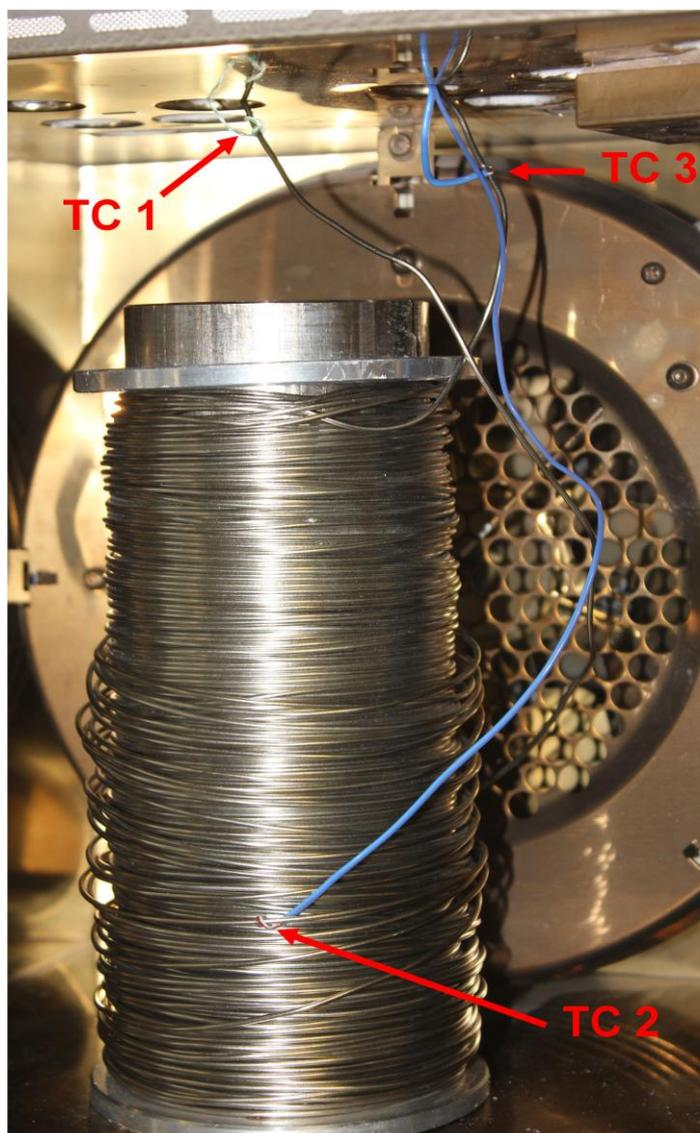
**Fig. S3:** Residence time unit (120 m stainless steel coil with an inner diameter of 0.8 mm) inside a GC-oven. To monitor the temperature at different positions thermocouples were installed at the entrance of the heated reaction zone (**TC 1**), after approximately 1 m of the coil (**TC 2**) and at the outlet of the oven (**TC 3**).
