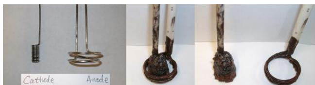
**Figure 14.** Vertical cylindrical configured electrodes used in the molten 730°C lithium carbonate electrolysis in which the cathode was placed inside the anode. Left, middle and right-hand photos respectively show the electrodes prior to the electrolysis, after electrolysis and after removal from the electrolyte, and finally after separation of the cathode from the anode.
