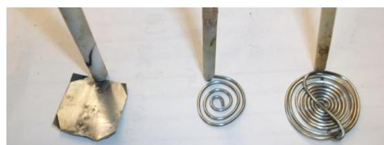
**Figure 8 (left).** Solid steel foil cathodes with various surface areas prior to electrolysis (top) and following electrolysis with partial removal of cathode product (bottom). Spot welds to connect the steel wire contacts are evident.
