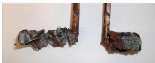
**Figure 18 (left).** Configuration: outer Ni anode is alumina tube shielded & inside is the coiled steel wire cathode.
