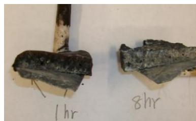
**Figure 6.** Product removed and partially peeled from cathode after 1 or 8 hour electrolyses. The amount of salt removed with the product is high after 1h electrolysis (then washed prior to analysis) & lower after the extended (8h) electrolysis. During the 8h electrolysis, a higher fraction of the initial 3 m of  $\text{Fe}^{3+}$  is converted to  $\text{Fe}^0$  & the product layer sitting on the cathode is enriched in iron metal.
