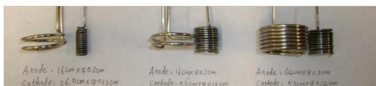
**Figure 17.** Vertical cylindrical configured, coiled electrodes with surface area varied by changing the length and coil diameter of the Ni (outer anode) or steel (inner cathode) wire as used in the molten 730°C lithium carbonate electrolysis.
