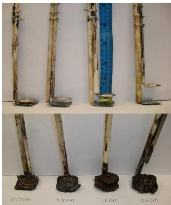
**Figure 2.** Anode (upper electrode) and cathode (lower electrode) prior to electrolysis (top) and following electrolysis prior to removal of cathode product (bottom). Insulating alumina ceramic tubes are reused and hence appear charred.
