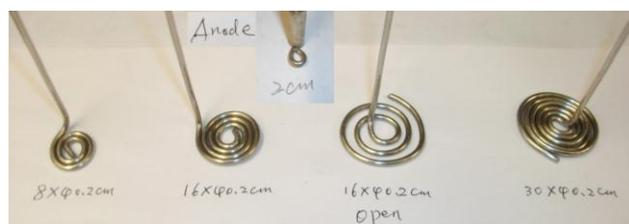
**Figure 11.** Coiled nickel wire anodes with a tight or loose (open) prior to the Table 12 electrolyses.
