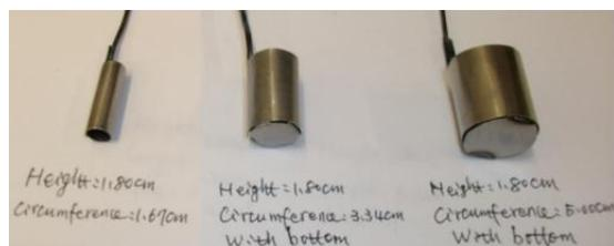
**Figure 20.** Vertical steel shim electrodes placed inside the anode for STEP Iron electrolysis as described in Table 21.
