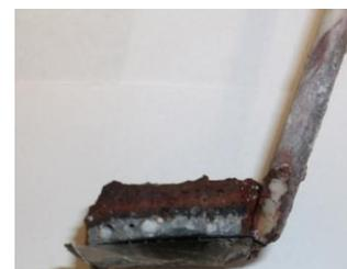
**Figure 7.** (right) Side view of cathode with product after 1h 3 m  $\text{LiFeO}_2$  in  $\text{Li}_{0.85}\text{Na}_{0.61}\text{K}_{0.54}\text{CO}_3$  750°C STEP iron electrolysis.
