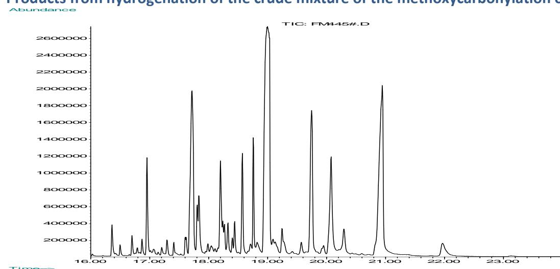
**"Methoxycarbonylation" of linoleic acid without CO (atmosphere of nitrogen)**
