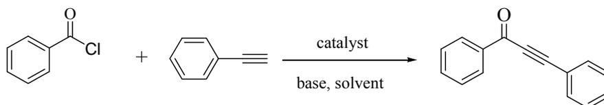
A oven-dried reaction tube was charged with catalyst, phenylacetylene (55 μL, 0.5 mmol), benzoyl chloride (87 μL, 0.75 mmol), base and solvent. The tube was sealed under nitrogen and was heated at 40 °C overnight. Then the reaction mixture was cooled and extracted with ethyl ether (3 × 10 mL). The yield of ynones were determined by GC analysis using dimethyl phthalate as an internal standard.
