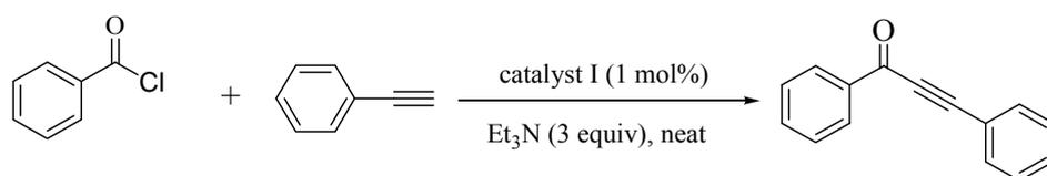
The reaction procedure was conducted as described above. After completion, the catalyst was separated by filtration, and the filtrate was followed by centrifugation. The two parts of residue were combined, dried and reused in the same reaction under identical conditions.
