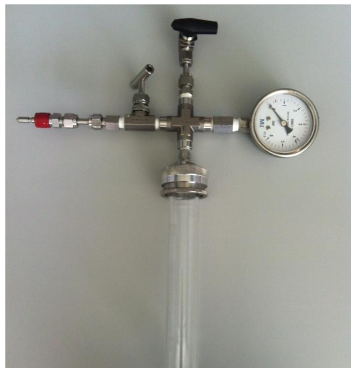
**Figure S9.** Schlenk reactor vessel.
