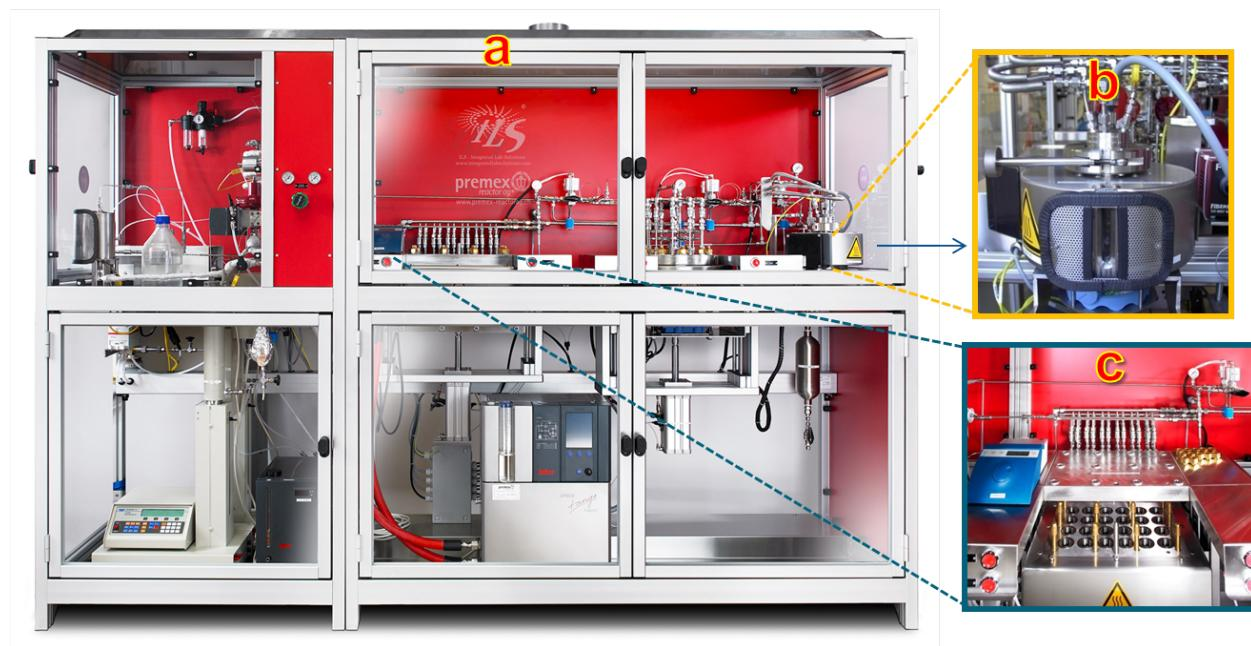
**Figure S2.** Supercritical CO<sub>2</sub> high-throughput platform used for the catalytic test (a): visualisation reactor (b) and 24 parallel batch reactors unit (c).
