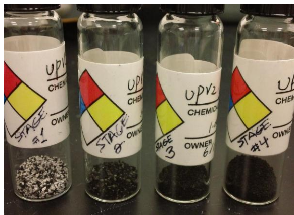
Fig. S6. Coked catalyst samples obtained from the microreactor experiments. The catalyst samples were collected at biomass-to-catalyst ratios: 0.4 (stage 1), 1.0 (stage 2), 1.7 (stage 3) and 5 (stage 4).
