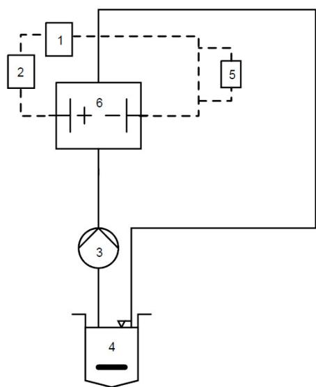
The electrochemical setup consisted of a storage vessel (4) from which the reaction solution was pumped with a peristaltic pump (3) through the electrochemical reaction cell (6) in a circular flow. A current was applied using a current generator (2) to enable hydrogen peroxide production catalyzed by a gas diffusion electrode (GDE). Current and voltage were measured with a series-connected digital ampere meter (1) and a parallel-connected voltmeter (5), respectively.
