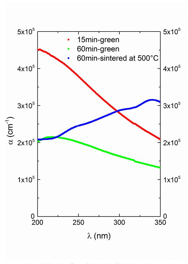
**Figure 13**. Linear optical absorption coefficients a of the as- deposited films during 15 min (red squares) and 60min (green squares) the film annealed at  $500^{\circ}$  C after depositing during 60min (blue squares) as a function of the wavelength  $\lambda$ .
