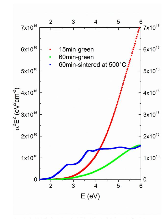
Figure 14. Plot of  $(\alpha h \upsilon)^2$  vs. hu for the as-deposited films during 15 min (red squares) and 60min (green squares) the film annealed at 500° C after depositing during 60min (blue squares). The optical band gap,  $E_g$ , is given by the intersection of the extrapolated linear section of the curve with the abscissa.
