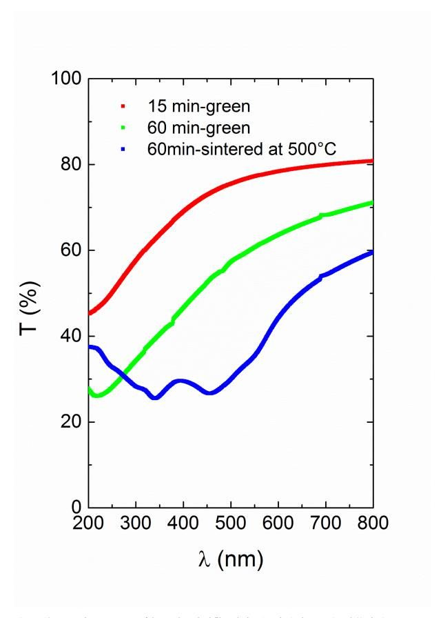
**Figure 12.** Transmittance spectra of the as- deposited films during 15 min (red squares) and 60min (green squares) the film annealed at 500° C after depositing during 60min (blue squares).
