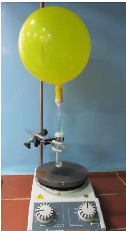
**Figure S2.** Reaction set-up without thermostatic control.
