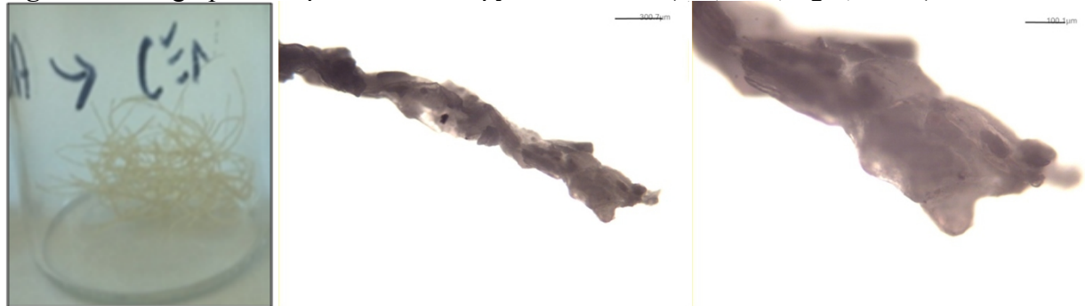
Fig. S3. Photograph and optical microscopy of CN fibers (left, 40X, right, 100X).
