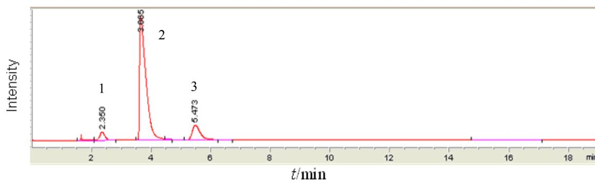
**Fig. S2** A typical GC spectrum of gas-phase products from oxidation of glucose in sodium metavanadate aqueous solution at 160°C. (1) CO<sub>2</sub>, (2) O<sub>2</sub>, (3) N<sub>2</sub>. N<sub>2</sub> was injected into the autoclave after reaction as the internal substance for quantification of CO<sub>2</sub>. O<sub>2</sub> was the residual after consumption in the reaction and CO<sub>2</sub> was produced in the reaction.
