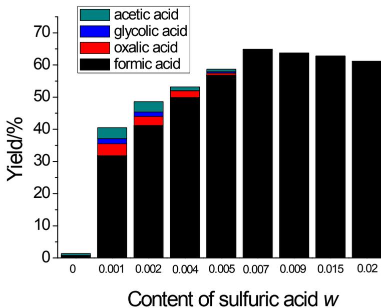
**Fig. S4** The distribution of products in liquid with cellulose as substrate as a function of sulfuric acid mass fraction  $w$ . Reaction conditions: cellulose, 100 mg; sodium metavanadate, 22 mg; water, 6 g; temperature, 160 °C; reaction time, 2 h.
