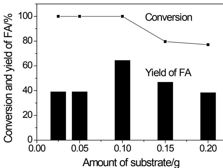
**Fig. S8** The effect of amount of initial substrate on the conversion of substrate and yield of FA. Reaction conditions: substrate, cellulose; sodium metavanadate, 22 mg; sulfuric acid, 42 mg; water, 6 g; temperature, 160 °C.
