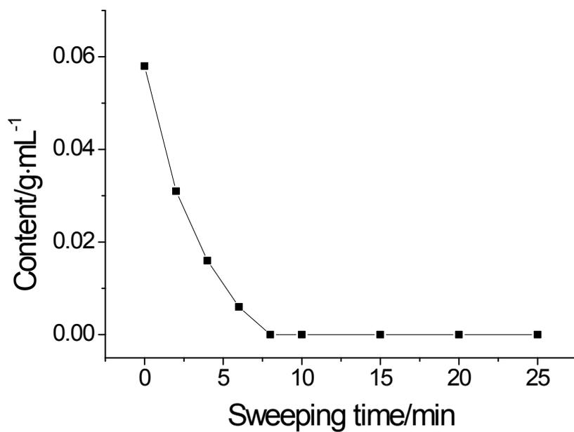
**Fig. S12** The content of diethyl ether in water after exhaustive extraction as a function of sweeping time. Sweeping gas, nitrogen; flowrate of nitrogen, 20 cm<sup>3</sup>/min; sweeping temperature, 30 °C.
