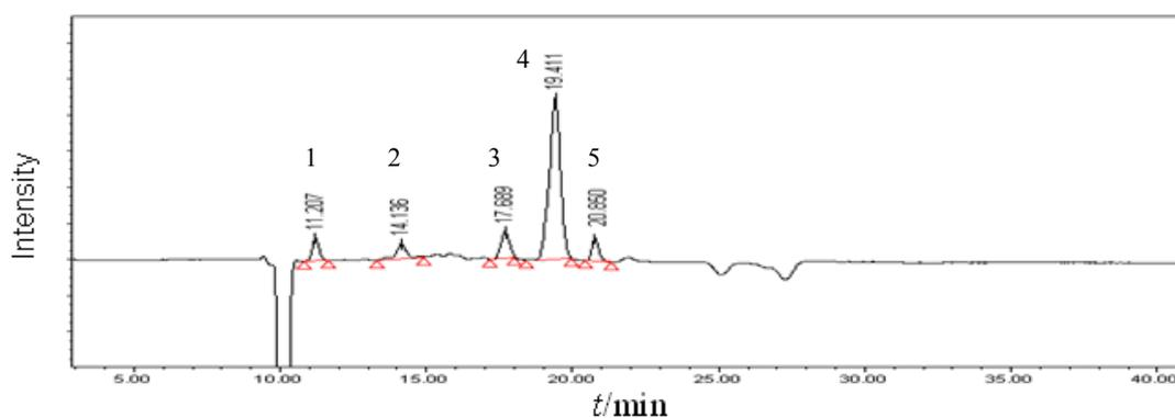
**Fig. S1** A typical HPLC spectrum of glucose oxidation products in sodium metavanadate aqueous solution at 160°C. (1) oxalic acid, (2) glucose, (3) glycolic acid, (4) formic acid, (5) acetic acid. The peak before the oxalic acid peak were caused by the mobile phase and was also observed in the standard sample. At times longer than the acetic acid peak, no additional peaks was observed.
