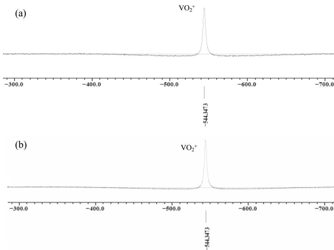
**Fig. S10**  $^{51}\text{V}$ -NMR spectras of the catalyst system before and after reaction (S1). (a), the catalyst system before reaction; (b), the catalyst system after reaction. Cellulose, 100 mg; sodium metavanadate, 22 mg;  $\text{H}_2\text{O}$ , 6 g;  $\text{H}_2\text{SO}_4$ , 42 mg ( $w = 0.007$ ); temperature,  $160\text{ }^\circ\text{C}$ ; reaction time, 2 h.
