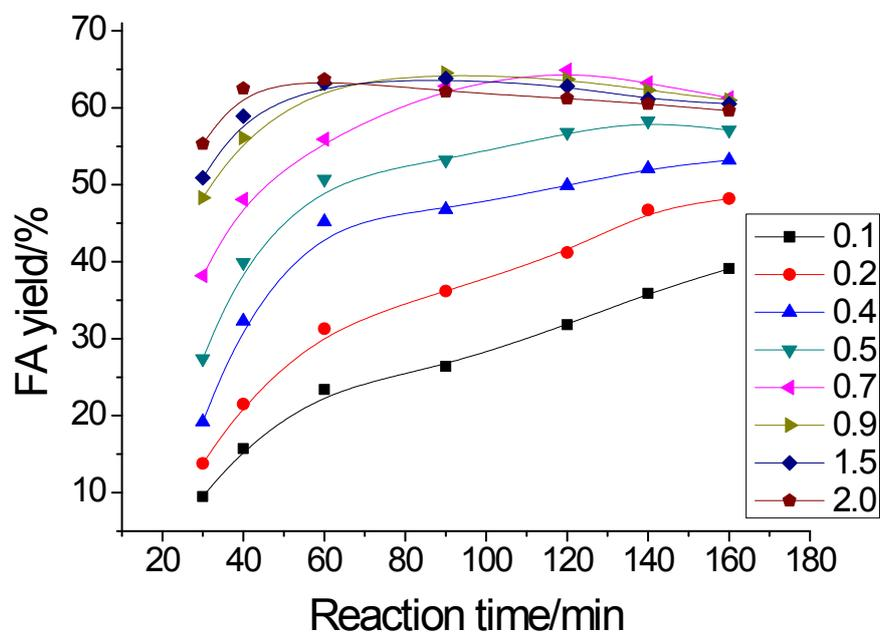
**Fig. S6** The yield of FA from cellulose as a function of time under different mass fractions of sulfuric acid 100w. Reaction conditions: cellulose, 100 mg; sodium metavanadate, 22 mg; water, 6 g; temperature, 160 °C.
