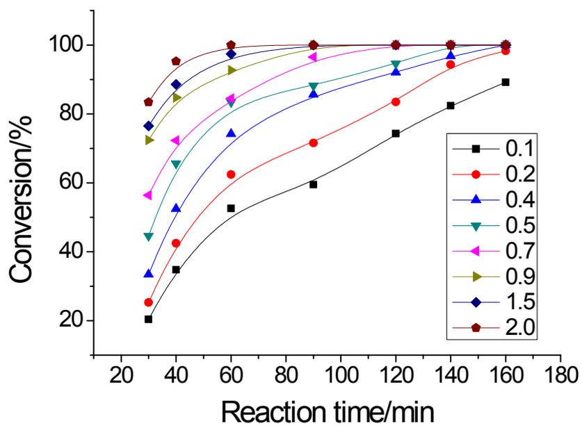
**Fig. S5** The conversion of cellulose as a function of time under different mass fractions of sulfuric acid 100w. Reaction conditions: cellulose, 100 mg; sodium metavanadate, 22 mg; water, 6 g; temperature, 160 °C.
