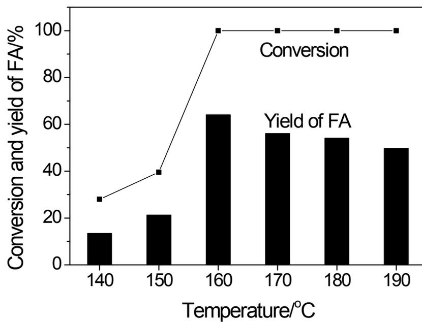
**Fig. S7** The effect of temperature on the conversion of substrate and yield of FA. Reaction conditions: cellulose, 100 mg; sodium metavanadate, 22 mg; sulfuric acid, 42 mg; water, 6 g.
