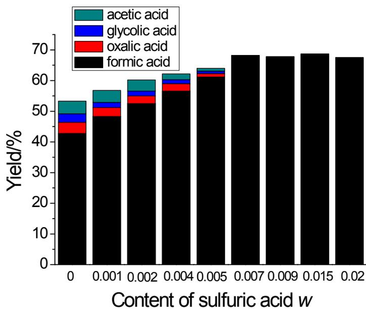
**Fig. S3** The distribution of products in liquid with glucose as substrate as a function of mass fraction of sulfuric acid *w*. Reaction conditions: glucose, 100 mg; sodium metavanadate, 22 mg; water, 6 g; temperature, 160 °C; reaction time, 1 min.
