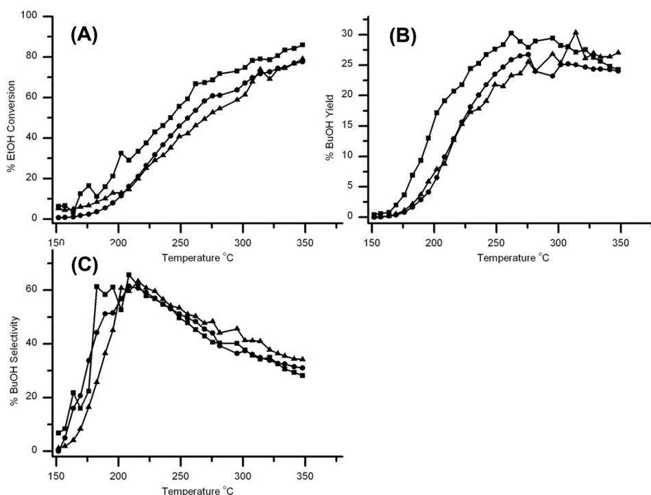
Figure S2 (A) EtOH conversion (B) BuOH yield (C) BuOH selectivity at different system pressures  $\blacktriangle$  70 bar,  $\blacksquare$  100bar and  $\bullet$  180 bar over Cu/HSACeO<sub>2</sub> in scCO<sub>2</sub>. System pressure has had little effect on the activity of the catalyst. Reaction conditions were as follows; 0.05 mL/ min EtOH, 1 mL/min CO<sub>2</sub>, 100 bar system pressure and temperature 150-350 °C at 0.3 °C/min.
