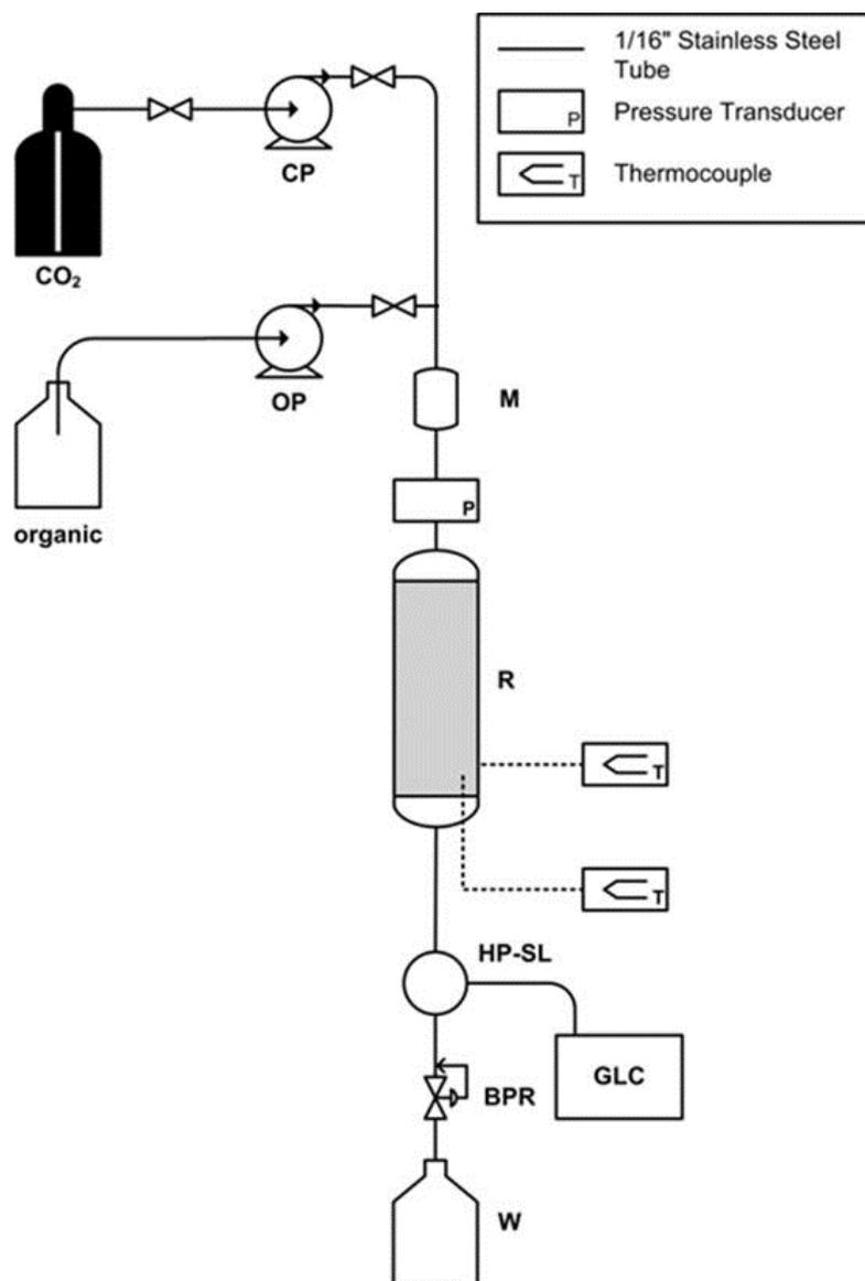
Figure S1. Schematic of flow reactor used for supercritical carbon dioxide reactions. The components are labelled as follows: CP, chilled CO<sub>2</sub> pump; M, mixer; OP, organic pump; PH, preheater and mixer; R, ¼ inch sand packed reactor containing Cu catalyst; HP-SL, high pressure sample loop; BPR, back pressure regulator; GLC, gas liquid chromatograph; W, organic waste.
