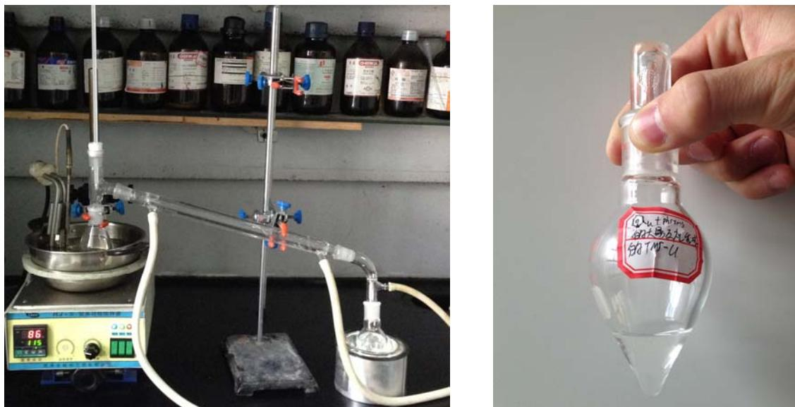
**Figure S1. Left:** the distillation apparatus; **Right:** freshly recovered  $\text{Me}_3\text{SiCl}$
