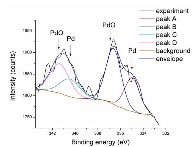
Figure 2. XPS spectrum of Pd 3d line taken from reused Pd-Fe nanocatalyst, sample 2. The expected line positions in the case of metallic Pd as well as of PdO are marked by arrows.
