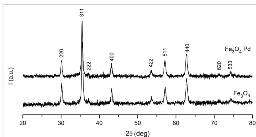
**Figure 1.** XRD pattern obtained from  $\text{Fe}_3\text{O}_4$  and Nanocat-Fe-Pd. All indexed lines correspond to cubic  $\text{Fe}_3\text{O}_4$  (JCPDS 75-1610).
