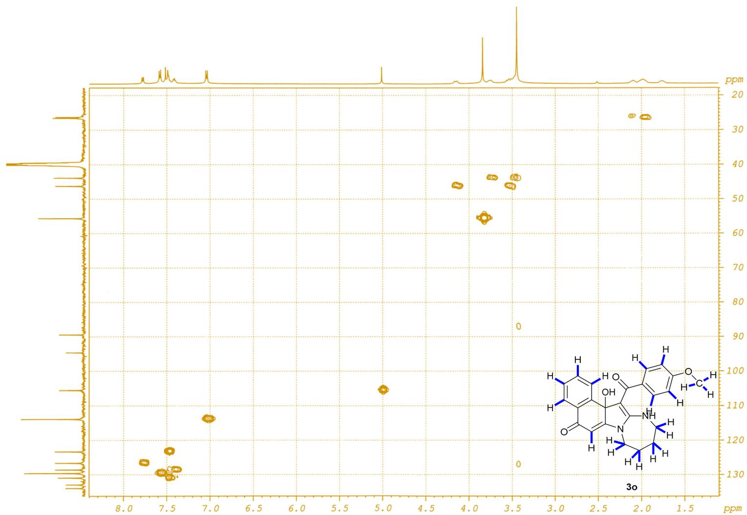
Fig. S50 HSQC (500 MHz, DMSO-*d*<sub>6</sub>) correlations (—) of compound 3o
