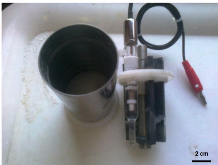
Supplementary Fig. 8. Images of employed electrochemical cell with 124 \text{ cm}^2 geometric area of working electrode.
