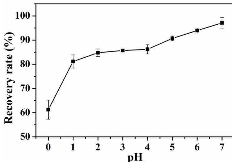
**Fig. S3** Recovery rate and adsorption efficiency of Au<sup>III</sup> by TP5.4 at different pH values. The HCl aqueous solution of Au<sup>III</sup> (1.5 g L<sup>-1</sup>, 1.0 mL) and TP5.4 (0.5 g L<sup>-1</sup>, 1.0 mL) were mixed at room temperature for 30 min.
