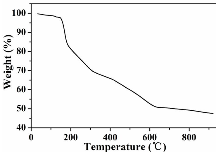
**Fig. S4** TGA of precipitate. The HCl aqueous solution ( $0.1 \text{ mol L}^{-1}$ ) of  $\text{Au}^{\text{III}}$  ( $1.5 \text{ g L}^{-1}$ ,  $1.0 \text{ mL}$ ) and TP5.4 ( $0.5 \text{ g L}^{-1}$ ,  $1.0 \text{ mL}$ ) were mixed at room temperature for 2 h. The precipitate was resuspended by distilled water and centrifuged ( $1000 \text{ g}$ ). The resultant precipitate was dried under vacuum before TGA analysis.
