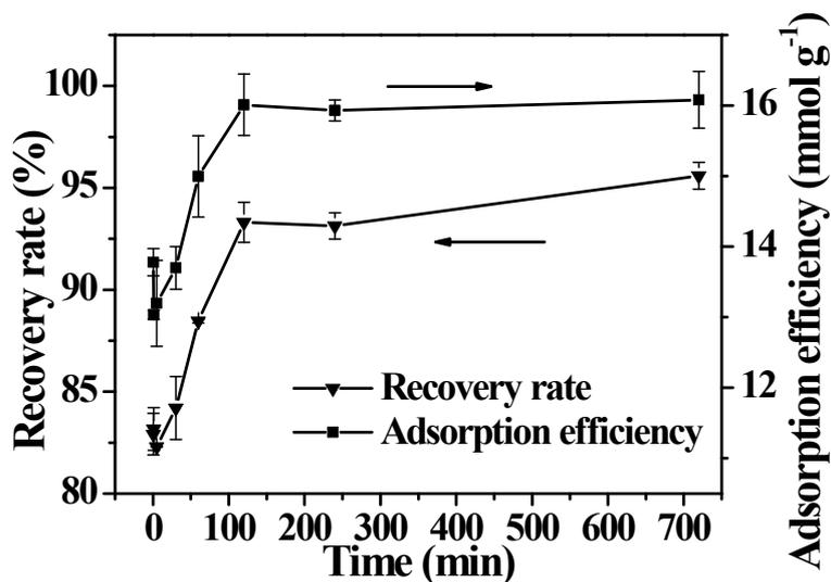
**Fig. S2** Recovery rate and adsorption efficiency of Au<sup>III</sup> by TP5.4 at different time points. The HCl aqueous solution (0.1 mol L<sup>-1</sup>) of Au<sup>III</sup> (1.5 g L<sup>-1</sup>, 1.0 mL) and TP5.4 (0.5 g L<sup>-1</sup>, 1.0 mL) were mixed at room temperature.
