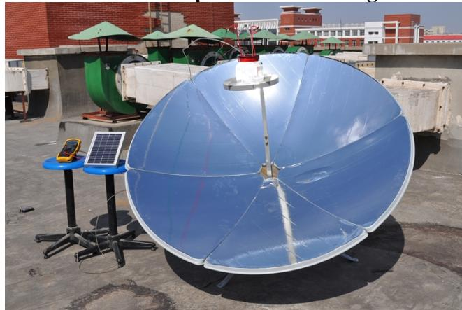
Outdoor STEP experimental apparatus. Individual components are detailed in reference 12. The photocurrent is generated by a silicon PV module, and under illumination yields an open circuit voltage: 21.8V; short circuit current ( $I_{sc}$ ): 0.2A; maximum power voltage ( $V_{mp}$ ): 18V; maximum power current( $I_{mp}$ ): 0.17A; maximum power ( $P_{max}$ ): 3W; solar efficiency: 18%.
