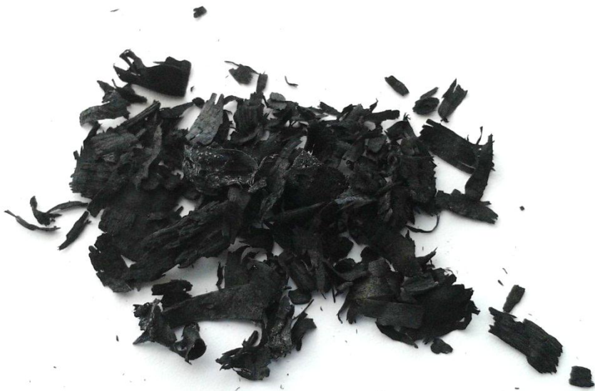
Figure S1 Photograph of the carbonized sawdust, showing individual flakes of wood have maintained their shape.
