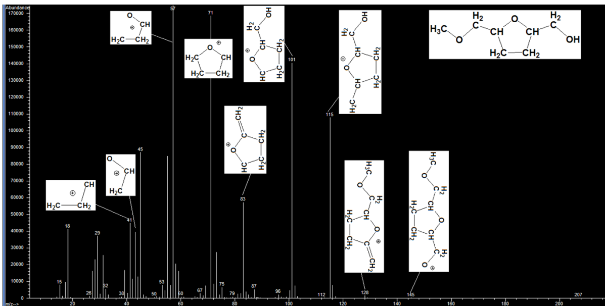
Figure S8 MS spectrum for tetrahydro-5-(methoxymethyl)furan-2-yl)methanol (THFM).
