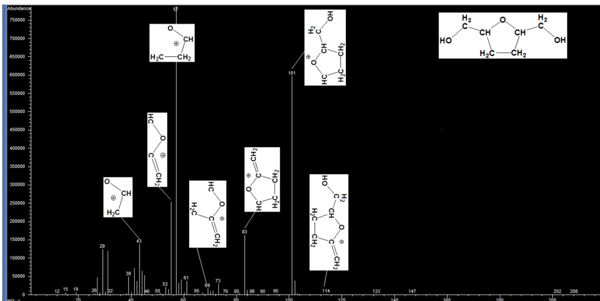
Figure S6 MS spectrum for cis-2,5-tetrahydrofurandimethanol (TFM).
