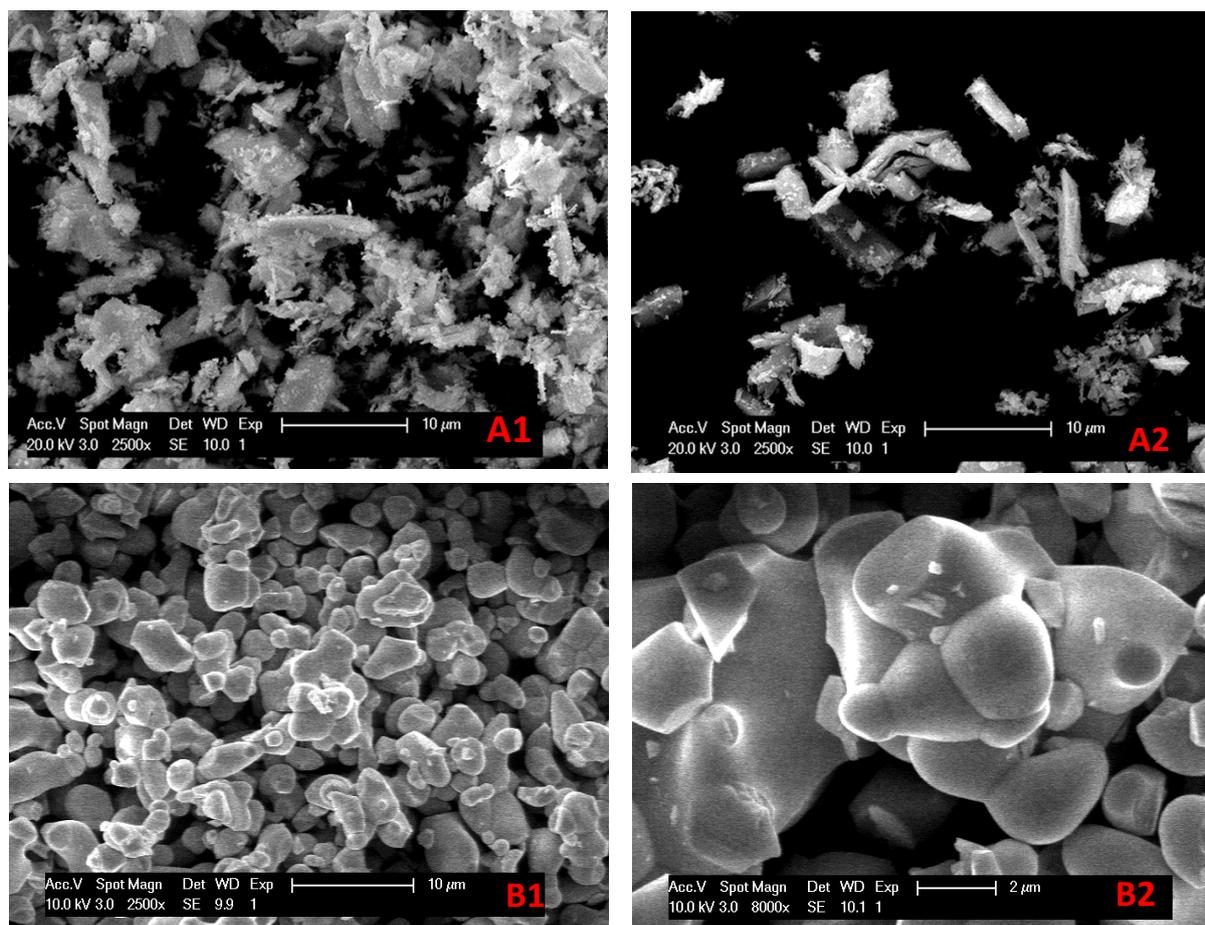
**Figure S1.** SEM images of the recycled YOX phosphor (A1, A2) and the purchased YOX phosphor (B1, B2). Image A1, A2 and B1 are magnified 2500 $\times$  and image B2 is magnified 8000 $\times$ .
