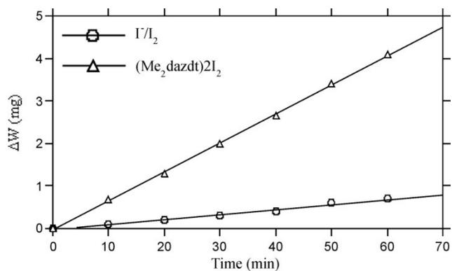
**Figure S7** - Plot of the gold weight loss  $\Delta W$  (mg) vs. the time (minutes) for calibrated wires of the same length and thickness dipped into equimolar solutions ( $c = 5.0 \times 10^{-3} \text{ mol dm}^{-3}$ ) of  $\text{Me}_2\text{dazdt}\cdot 2\text{I}_2$  adducts in THF and  $\text{I}_2/\text{KI}$  in water.
