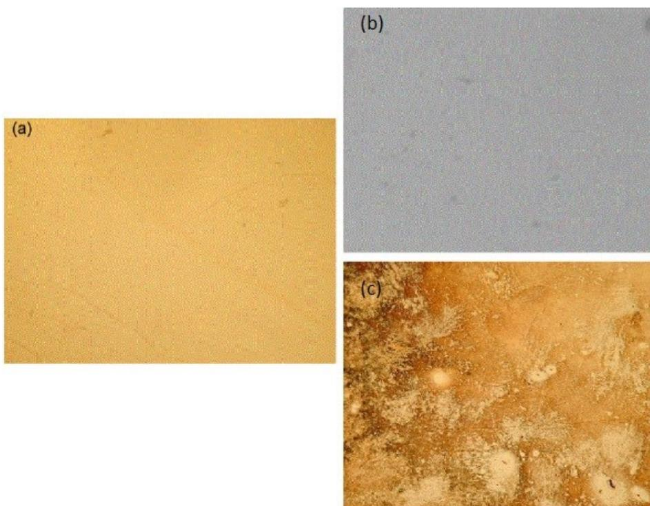
**Figure S8** - Si/SiO<sub>2</sub>/Ti/Au thin layers before (a) and after 5' of etch by  $\text{Me}_2\text{dazdt}\cdot 2\text{I}_2$  THF solution (b), and  $\text{I}_2/\text{I}^-$  water solution (c).  $c = 5.0 \times 10^{-3} \text{ mol L}^{-1}$ .
