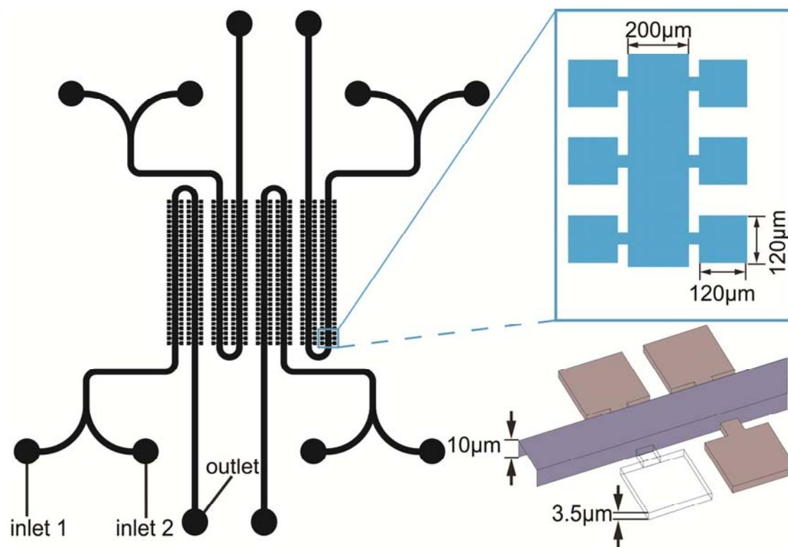
**Figure S1.** The chip layout planar graph and 3D structure. **Left**, the profile of the microfluidic chips used in this work. **Top right**, the dimensions of the main channels and the growth chambers. **Bottom right**, the 3D structures and vertical dimensions of the main channels and the growth chambers.
