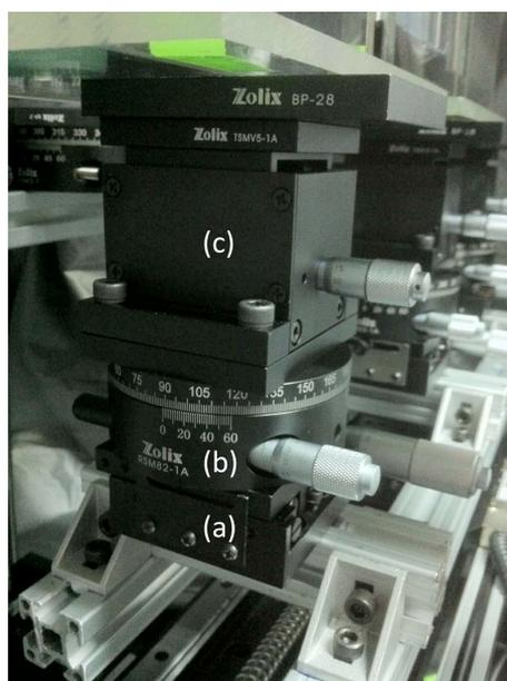
**Fig. S1** Three horizontal (TSM25-1A, Zolix Instrument, Beijing, China), rotational (RSM82-1A, Zolix Instrument, Beijing, China), and vertical (TSMV5-1A, Zolix Instrument, Beijing, China) stages that hold the sample chambers are shown in the figure as (a), (b), and (c), respectively. The stages are constructed vertically, and fixed on the automated translational stage by aluminum frame.
