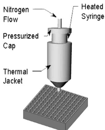
**Fig. S1** Well system fabrication. Free form fabrication with 3D-plotters. Material extrusion occurred by nitrogen pressure. Wells are rectangular, with closed bottom and sides, and opened top. The strand distance is defined by the symmetrical space between one well wall and one well (empty space) and repeated throughout the device.
