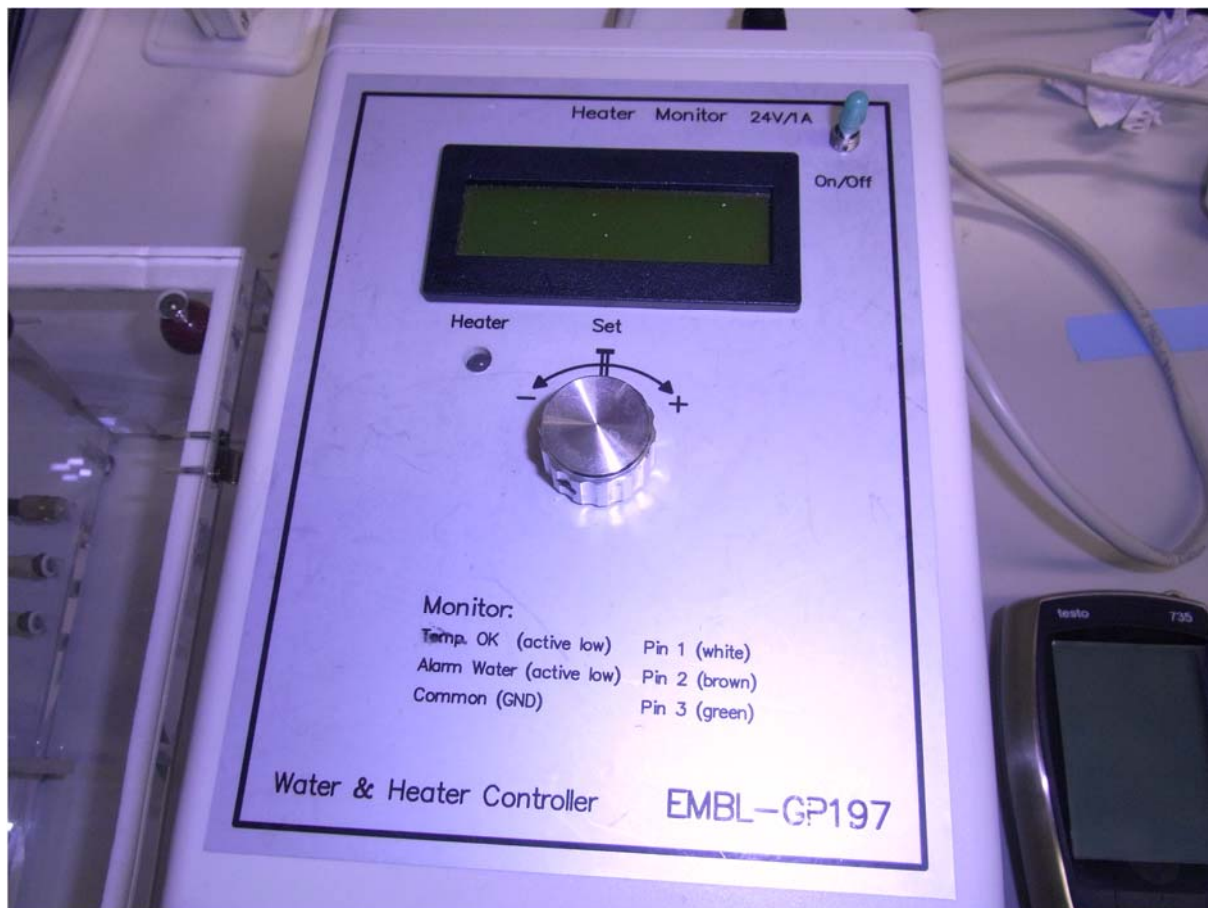
Figure 5 – EMBL-GP197 heating controller.
