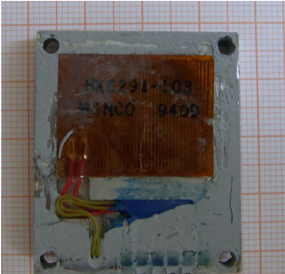
Figure 4 – Heating foil mounted in the heating plate.
