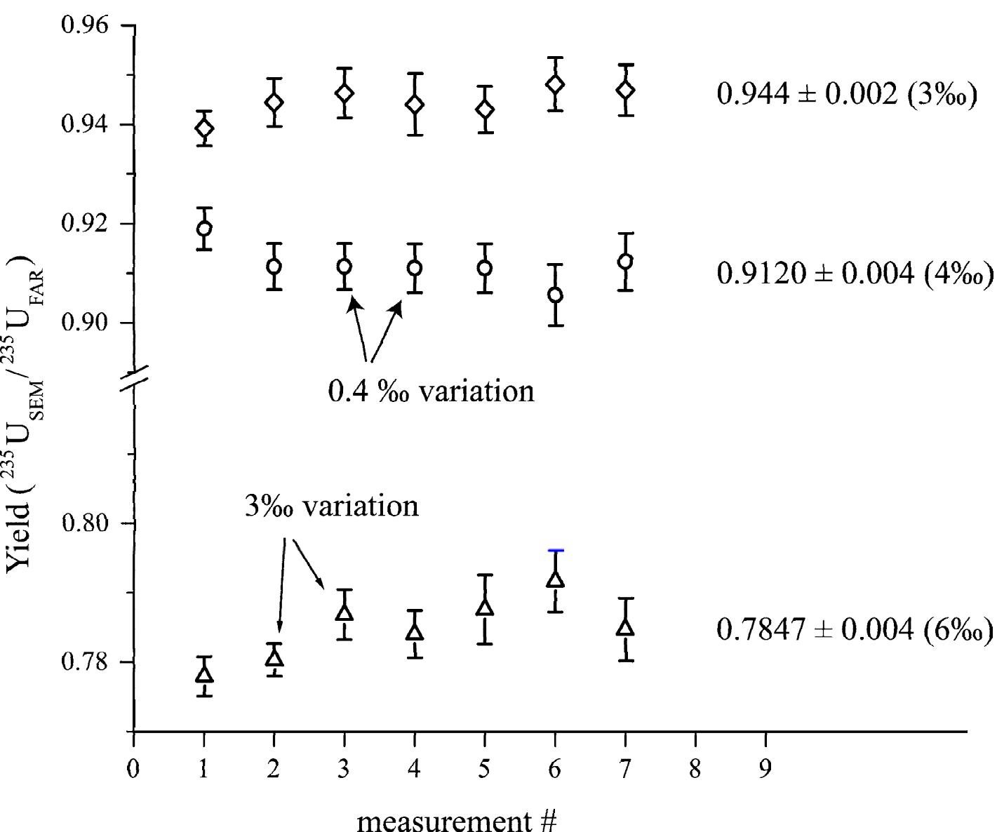
Stability of the calculated  $^{235}\text{U}$  SEM/FAR yield for three different sessions. Data corresponds to ion beam intensities ranging between 0.3 and 0.6 V. Arrows indicate maximum and minimum variability.
