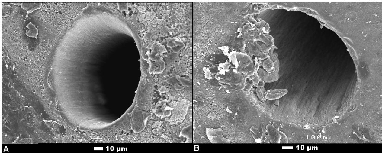
Figure 1. A. SEM image of ablation crater in xerogel. B. Showing spalling. Surface non-orthogonal to image
