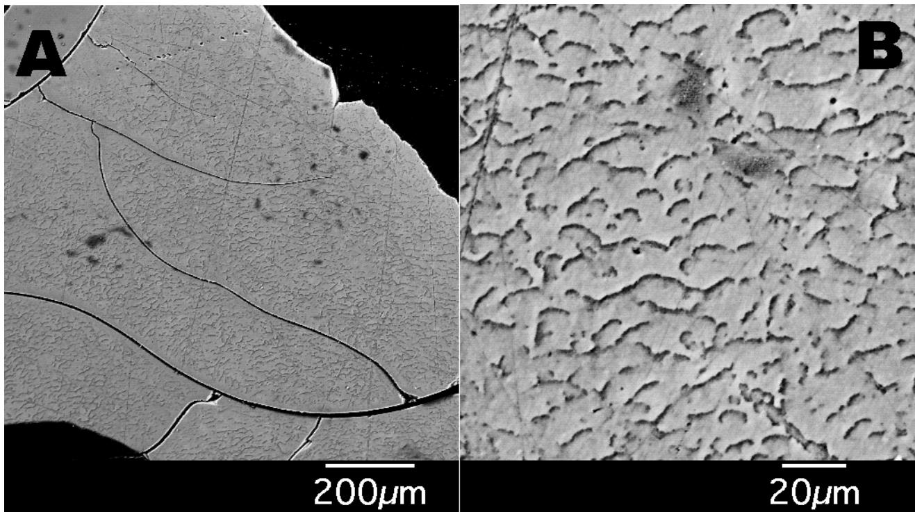
Figure 2. Electron backscatter images of xerogels. Darker patches in upper centre of B are thinner portions of the thin section (also observed under optical microscopy). Linear features are of topographic origin
