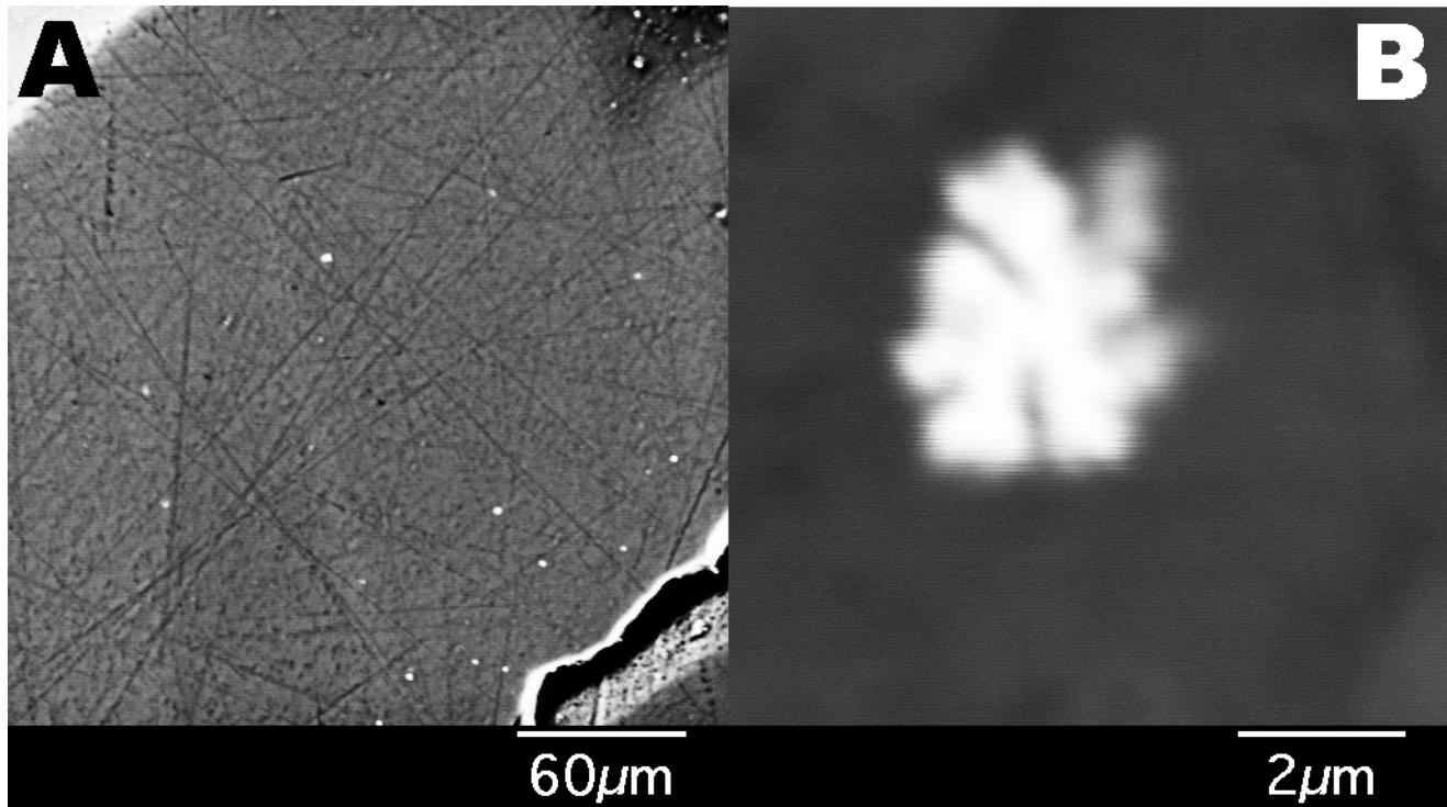
Figure 3. Electron backscatter image of series 5 xerogel (SG5A) with selenium, sulphur and metal rich inclusions [bright spots] (A), with close-up of inclusions (B)
