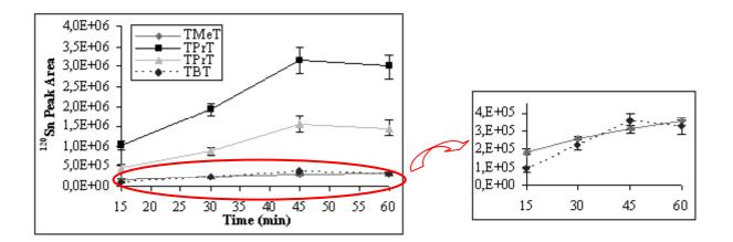
**Fig. S2**. Effect of extraction time on the chromatographic response. The fiber was exposed to samples containing 5  $\mu$ g L<sup>-1</sup> of each compound as Sn and 75 g L<sup>-1</sup> of NaCl. Each point is the average of the three data points.
