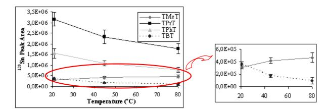
**Fig. S3**. Effect of temperature on extraction efficiency. The fiber was exposed to samples containing 5  $\mu$ g L<sup>-1</sup> of each compound as Sn and 75 g L<sup>-1</sup> of NaCl. Each point is the average of the three data points.
