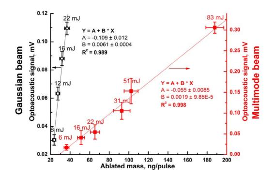
Fig. S1 Optoacoustic signal as a function of ablated mass.
