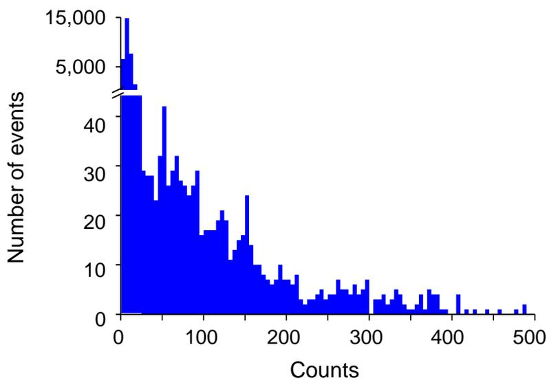
Fig. II (ESI): Histogram of measured  $^{57}\text{Fe}^+$  ion signal intensities. (0.05 cell/drop; sample integration time: 1 ms; counting mode. Histogram calculated for intensity intervals of 5 counts. Number of runs: 400).
