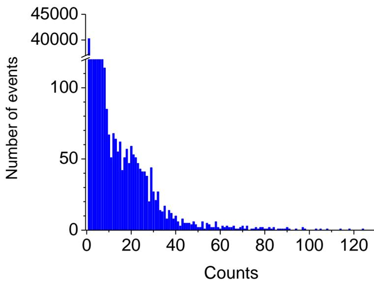
Fig. I b (ESI) Histogram of measured  $^{25}\text{Mg}^+$  ion signal intensities. (0.01 cell/drop; sample integration time: 1 ms; counting mode. Histogram calculated for intensity intervals of 1 counts. Number of runs: 2000).
