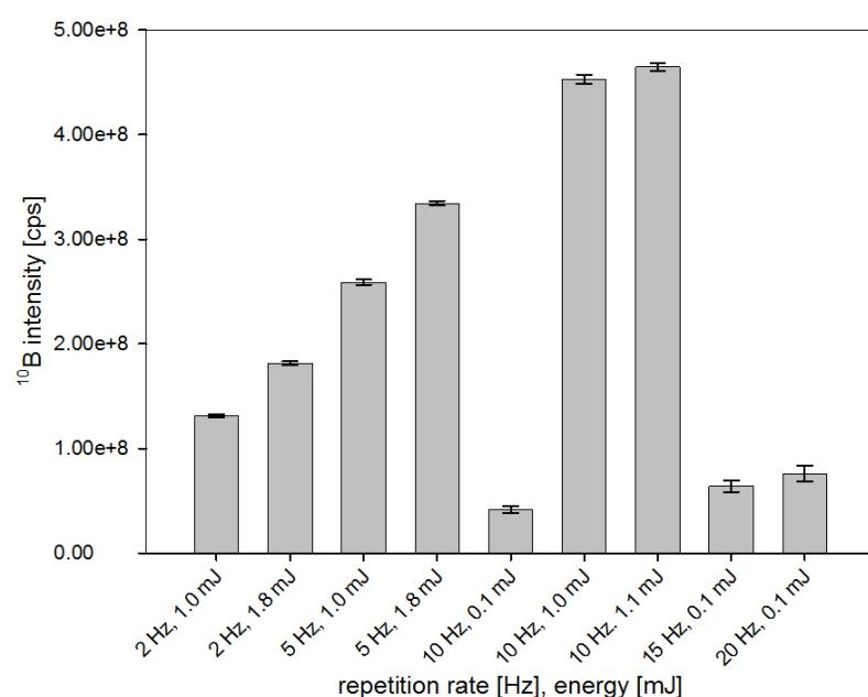
**Figure 12** Optimization of laser parameters: Comparison of  $^{10}\text{B}$  intensity (S97 IRM) with different repetition rate (2 – 20 Hz) and different laser energy (0.1 – 1.8 mJ) at constant spot size (200  $\mu\text{m}$ ) using fs-LA (Legend, Coherent Inc., USA) and MC-ICPMS (Nu Plasma HR MC-ICPMS, Nu Instruments, Wrexham, Great Britain)
