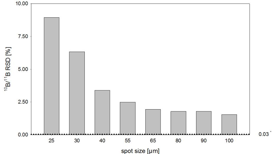
**Figure 9** Optimization of laser parameters: Comparison of  $^{10}\text{B}/^{11}\text{B}$  relative standard deviation (RSD) (IRM S97) with different spot size (25 - 100  $\mu\text{m}$ ) constant repetition rate (5 Hz) and 60 % laser energy ( $0.5 \text{ J cm}^{-2}$ ) using ns-LA (UP-213, New Wave Research, Fremont, CA, USA) and Q-ICPMS (Agilent 7700x quadrupole ICPMS, Agilent Technologies, Waldbronn, Germany)
