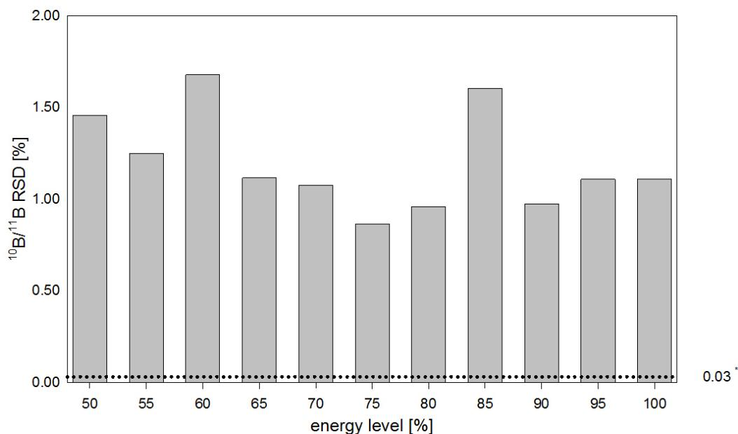
**Figure 5** Optimization of laser parameters: Comparison of  $^{10}\text{B}/^{11}\text{B}$  relative standard deviation (RSD) (IRM S97) with different laser energy levels (50 - 100 %) at constant spot size (100  $\mu\text{m}$ ) and repetition rate (10 Hz) using ns-LA (UP-213, New Wave Research, Fremont, CA, USA) and Q-ICPMS (Agilent 7700x quadrupole ICPMS, Agilent Technologies, Waldbronn, Germany)
