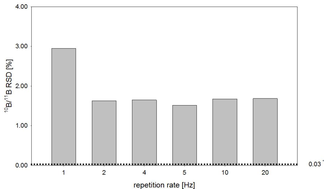
**Figure 7** Optimization of laser parameters: Comparison of  $^{10}\text{B}/^{11}\text{B}$  relative standard deviation (RSD) (IRM S97) with different repetition rate (1 - 20 Hz) at constant spot size ( $100\ \mu\text{m}$ ) and 60 % laser energy ( $0.5\ \text{J cm}^{-2}$ ) using ns-LA (UP-213, New Wave Research, Fremont, CA, USA) and Q-ICPMS (Agilent 7700x quadrupole ICPMS, Agilent Technologies, Waldbronn, Germany)
