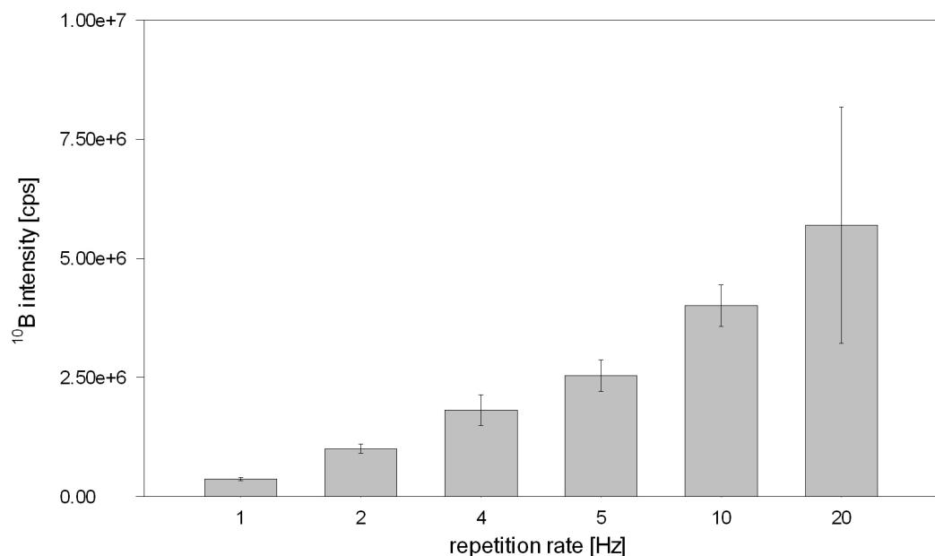
**Figure 6** Optimization of laser parameters: Comparison of  $^{10}\text{B}$  intensity (IRM S97) with different repetition rate (1 - 20 Hz) at constant spot size (100  $\mu\text{m}$ ) and 60 % laser energy (0.5  $\text{J cm}^{-2}$ ) using ns-LA (UP-213, New Wave Research, Fremont, CA, USA) and Q-ICPMS (Agilent 7700x quadrupole ICPMS, Agilent Technologies, Waldbronn, Germany)
