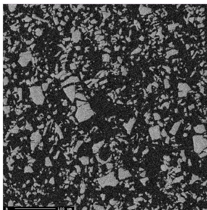
**Figure 2** Boron distribution in IRM in house reference material S97, recorded by EPMA (B K $\alpha$  line at 129.29 nm on a layered dispersion element (LDEB) diffracting crystal-) - mapping size 512 x 512  $\mu\text{m}$  – light areas indicate high boron content (JXA-8200 Superprobe, JEOL, Tokyo, Japan)
