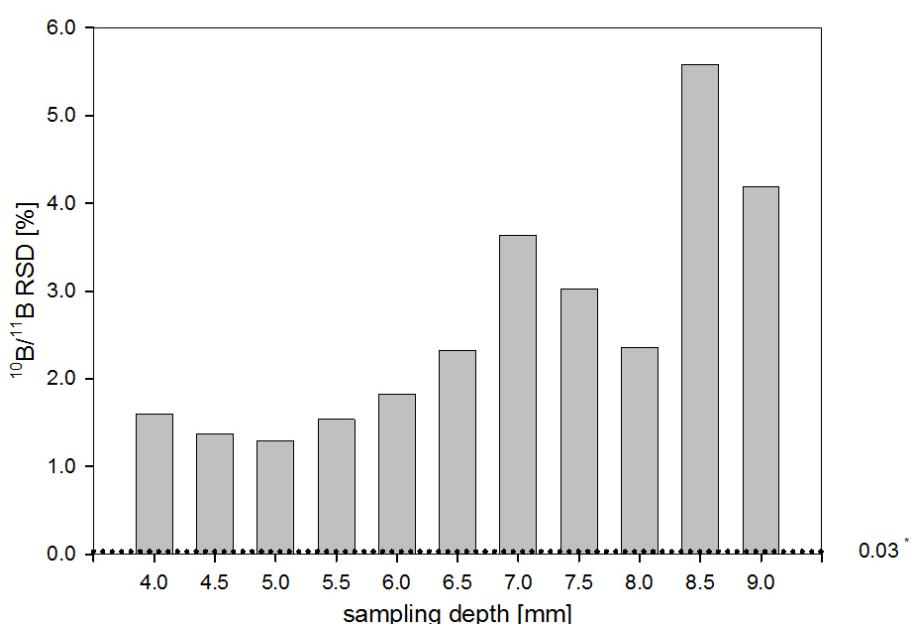
**Figure 11** Optimization of ICPMS parameters: Comparison of  $^{10}\text{B}/^{11}\text{B}$  relative standard deviation (RSD) (IRM S97) with different sampling depth (4.0 - 9.0 mm) using Q-ICPMS (Agilent 7700x quadrupole ICPMS, Agilent Technologies, Waldbronn, Germany) at constant laser ablation settings (ns-LA, 100  $\mu\text{m}$ , 0.5  $\text{J cm}^{-2}$ , 5 Hz)
