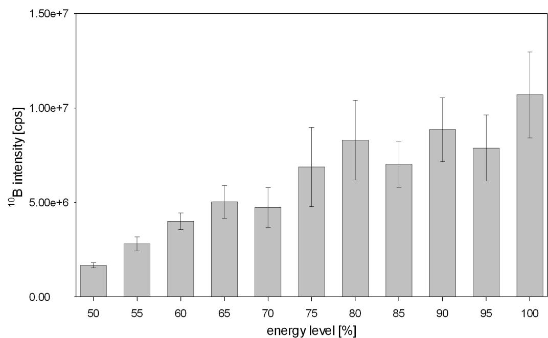
**Figure 4** Optimization of laser parameters: Comparison of  $^{10}\text{B}$  intensity (IRM S97) with different laser energy levels (50 – 100 %) at constant spot size (100  $\mu\text{m}$ ) and repetition rate (10 Hz) using ns-LA (UP-213, New Wave Research, Fremont, CA, USA) and Q-ICPMS (Agilent 7700x quadrupole ICPMS, Agilent Technologies, Waldbronn, Germany)
