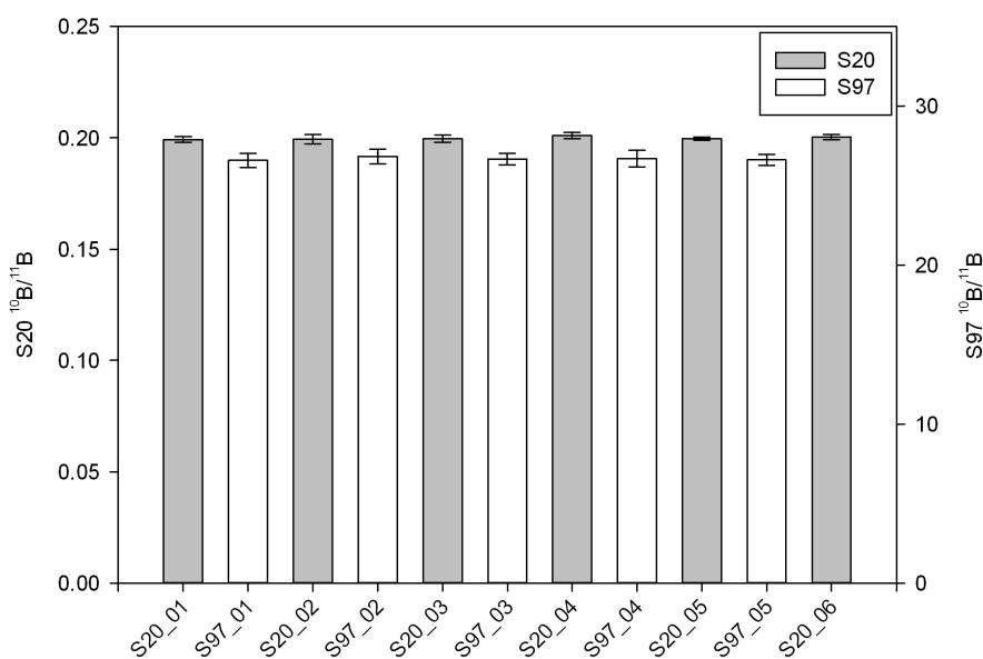
**Figure 14** Measurement sequence for mass bias correction of IRM S97 using IRM S20 as standard (ns-LA-ICPMS). The arithmetic mean of two IRM S20 values is used to correct the IRM S97 value in the middle.
