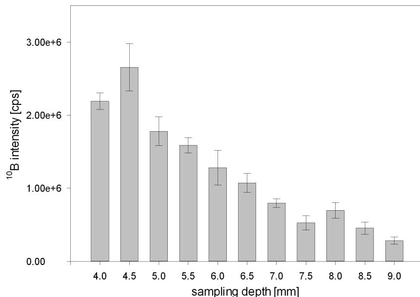
**Figure 10** Optimization of ICPMS parameters: Comparison of  $^{10}\text{B}$  intensity (IRM S97) with different sampling depth (4.0 - 9.0 mm) using Q-ICPMS (Agilent 7700x quadrupole ICPMS, Agilent Technologies, Waldbronn, Germany) at constant laser ablation settings (ns-LA, 100  $\mu\text{m}$ ,  $0.5 \text{ J cm}^{-2}$ , 5 Hz)
