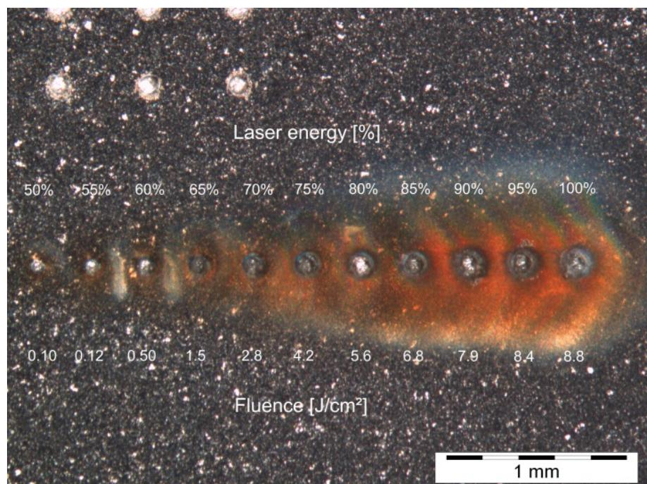
**Figure 3** Light microscope picture of 100  $\mu\text{m}$  ablation spots by ns-LA-ICPMS with increasing energy level (50 – 100 % or 0.10 – 8.8  $\text{J cm}^{-2}$ ) at constant repetition rate (10 Hz) on IRM in-house reference material S97 – higher energy leads to more deposition on the sample
