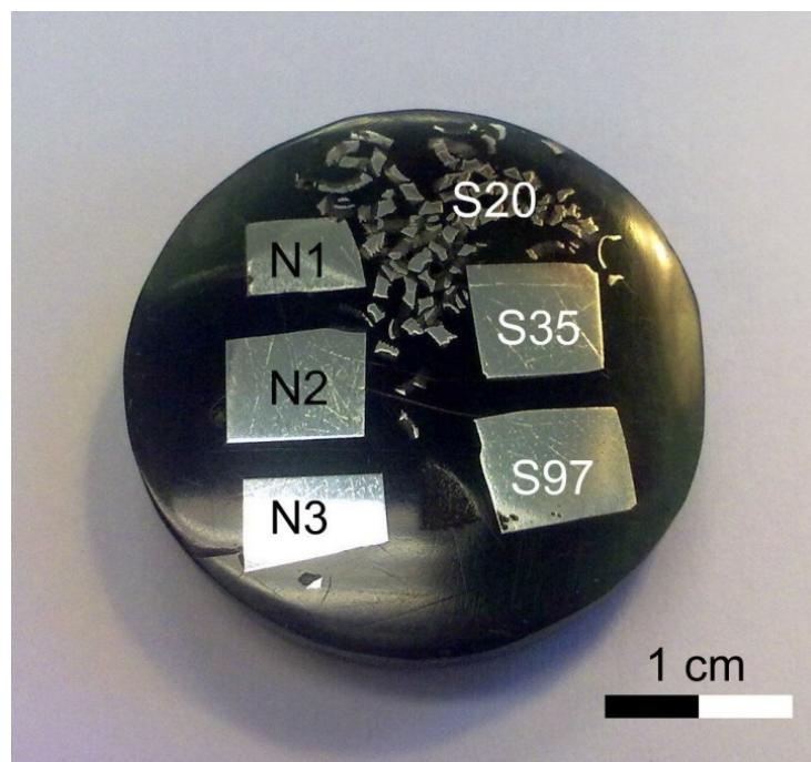
**Figure 1** IRM In-house reference materials S20 (metal chips), S35, S97, and process samples N1, N2 and N3 cast in a one inch mold with epoxy resin, polished and ready for EPMA and LA-ICPMS analysis
