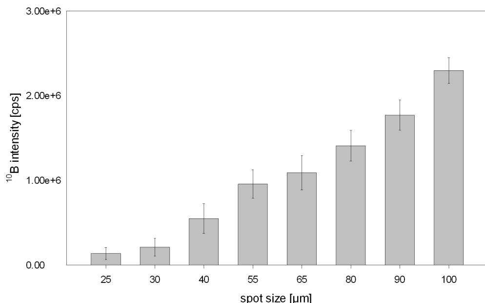
**Figure 8** Optimization of laser parameters: Comparison of  $^{10}\text{B}$  intensity (IRM S97) with different spot size (25 - 100  $\mu\text{m}$ ) at constant repetition rate (5 Hz) and 60 % laser energy ( $0.5\ \text{J cm}^{-2}$ ) using ns-LA (UP-213, New Wave Research, Fremont, CA, USA) and Q-ICPMS (Agilent 7700x quadrupole ICPMS, Agilent Technologies, Waldbronn, Germany)
