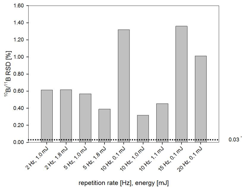
**Figure 13** Optimization of laser parameters: Comparison of  $^{10}\text{B}/^{11}\text{B}$  relative standard deviation (RSD) (IRM S97) with different repetition rate (2 - 20 Hz) and different laser energy (0.1 - 1.8 mJ) at constant spot size (200  $\mu\text{m}$ ) using fs-LA (Legend, Coherent Inc., USA) and MC-ICPMS (Nu Plasma HR MC-ICPMS, Nu Instruments, Wrexham, Great Britain)
