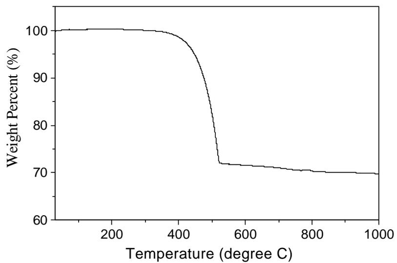
**Figure S2** TGA curve of sample I under Ar atmosphere.
