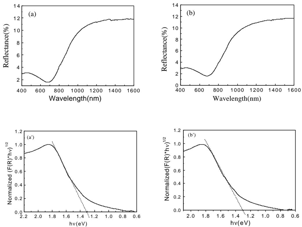
**Figure S3** DRS of the sample I ((a)) and III ((b)); the normalized plots of  $(F(R) \cdot hv)^{1/2}$  versus  $hv$  (eV) ((a') and (b')) corresponding to the data deriving from spectra (a) and (b).
