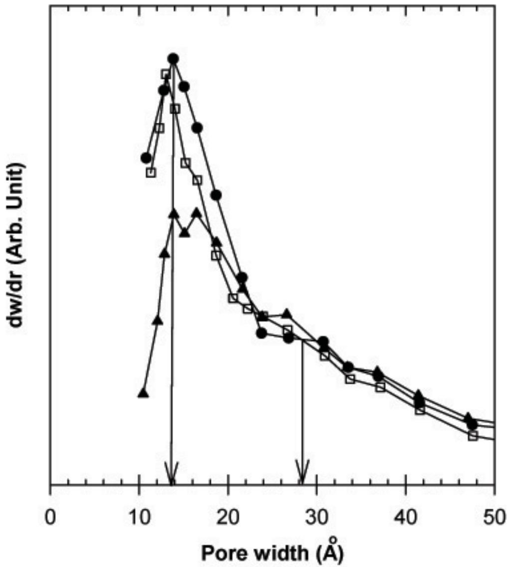
BJH pore-size distribution for  $\text{SiO}_2/\text{ZrO}_2$  sol-pillared clay dependent on calcination temperature. SZPC-300 (open squares), SZPC-400 (closed circles), and SZPC-500 (closed triangles).
