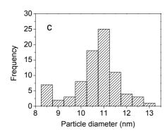
The size distribution of samples (a) modified with TOPO and PVP, (b) modified with HDA and PVP, (c) modified with PVP only.
