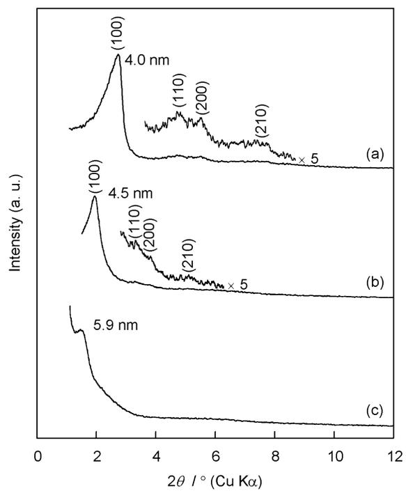
**Figure S1.** XRD patterns of (a) APW-2 and BTSE-modified mesostructured AlPO-based materials obtained where the Si/(Al+P) molar ratios were (b) 0.25 and (c) 0.50.
