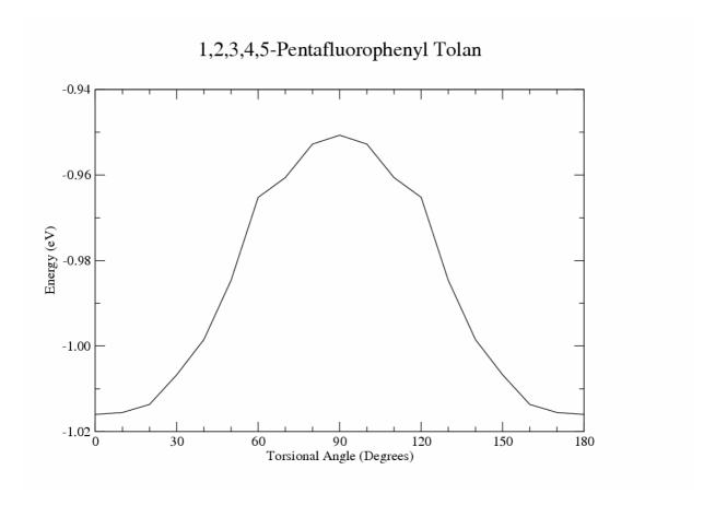
Figure S1: Energy as a function of inter-ring torsion angle in 1,2,3,4,5-pentafluoro tolan.
